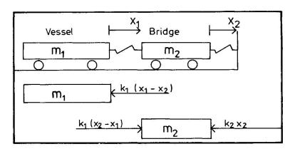
By means of the connections presented in Figure 5, the following equations of equilibrium are obtained:
