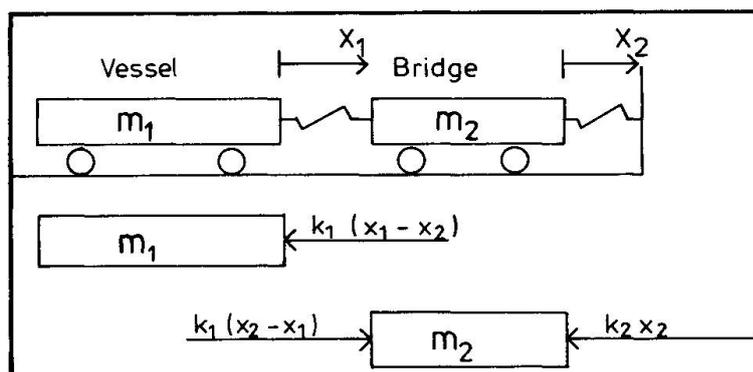
By means of the connections presented in Figure 5, the following equations of equilibrium are obtained:
