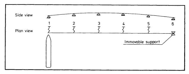
Figure 3. Construction model in a collision.
