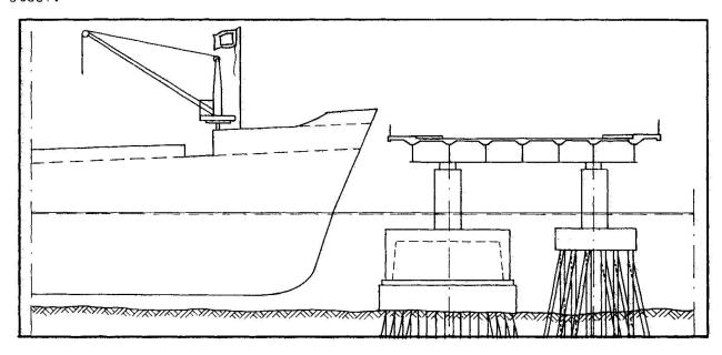
Figure 2. Bridge cross-section and the bow of a coal-carrying ship.
