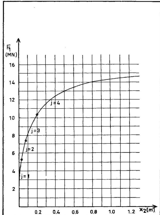
Figure 7. Curve of contact force - displacement
