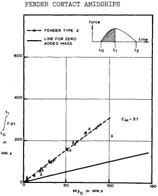
Fig. 5 Impulse versus change of momentum during compression phase
