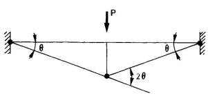
Fig. 2 Collapse mechanism for bracing
