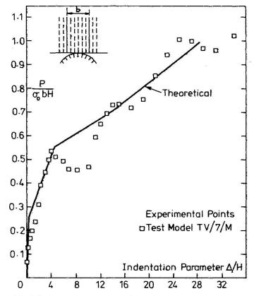
Fig. 3 (e) Comparison of Experimental and Theoretical Results: TV/7/M
