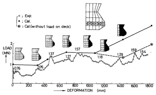
Fig.6 Load-deformation curve of tanker model
