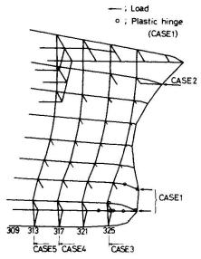
Fig. 7 Idealized model of container carrier
