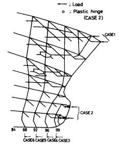
Fig.9 Idealized model of ice strengthend ship
