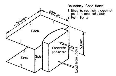
Fig.1 Overall dimensions of Typical Test Model and Loading Scheme
