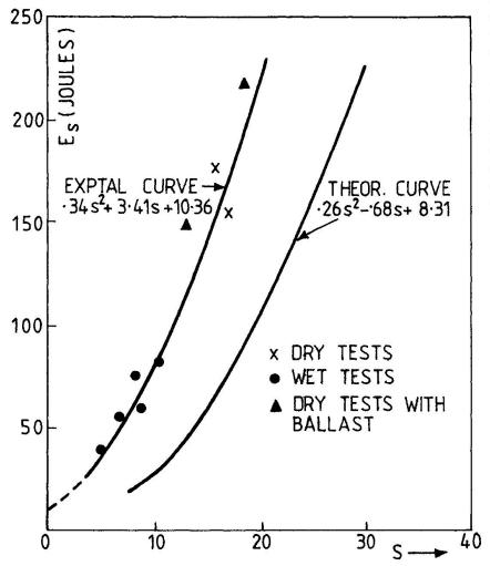
deflections greater than eight times the plate thickness, the permanent set was dictated by the energy of the striker. This led to a permanent set versus energy relationship that could be accurately represented by a parabola. The curve is shown in Fig.3 together with an expression which describes the parabola.
