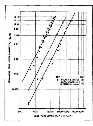
Fig. 3 Dependence of dent depth on lateral load
