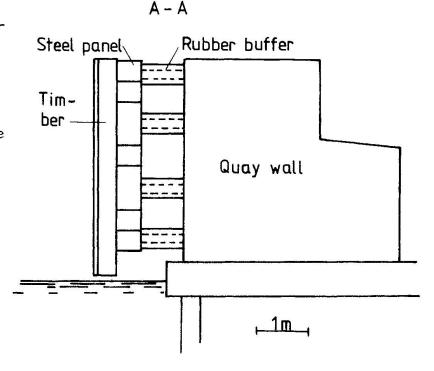
Fig.3 Fender constructions in Korsør ferry harbour.
