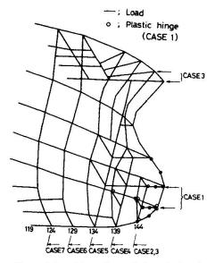
Fig.8 Idealized model of tanker
