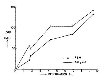
Fig.10 Load-deformation curve of container carrier by FEM
