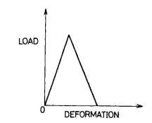
Fig.1 Load-deformation curve of longitudinal member
