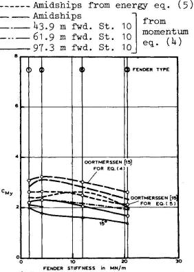
Fig. 6 C<sub>My</sub> obtained from energy and momentum balance (eq. (5) and (4)) over compression phase
