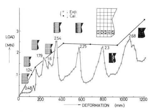
Fig.5 Load-deformation curve of container carrier model
