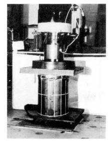
Fig. 7 Initial buckling of model in Fig. 6
