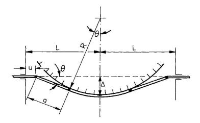
Fig. 4 Beam Loaded through a Circular Indenter
