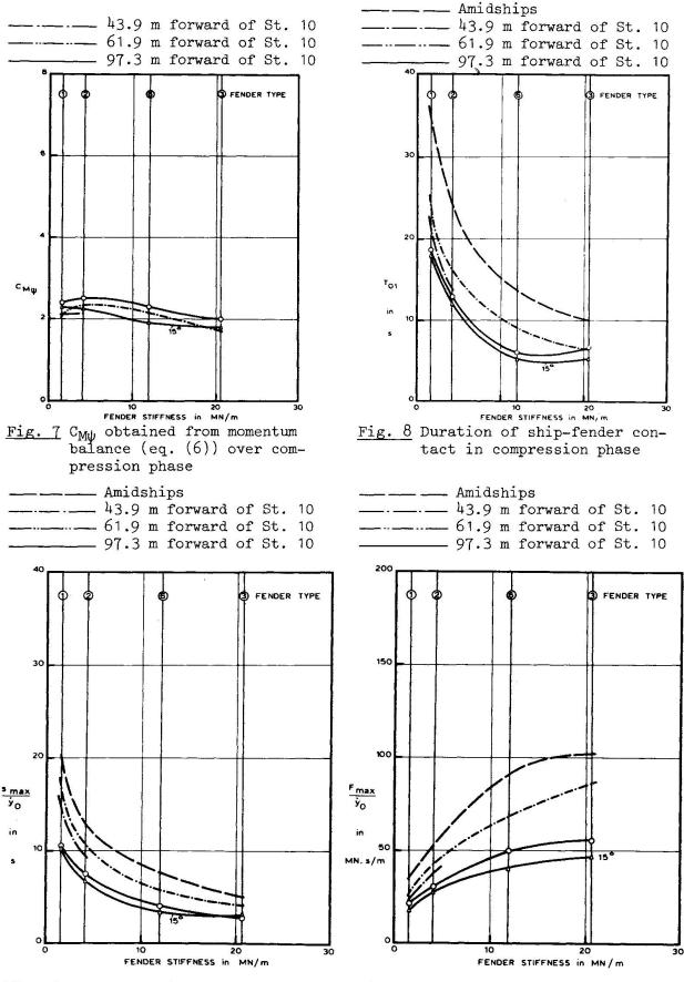
Fig. 9 Reduced maximum fender deflection
