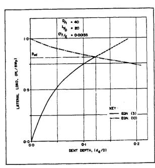
Fig. 4 Estimation of ultimate lateral load, Pud
