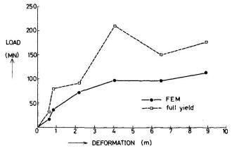
Fig.12 Load-deformation curve of ice strengthend ship
