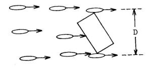
Nau =  $\rho$  VDT  $\cdot \cdot \cdot (1)$  Fig. 1 Collision with fixed object
