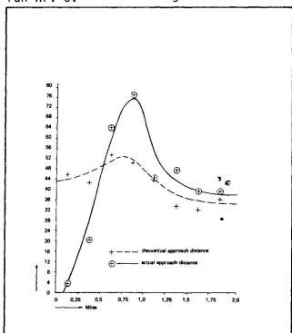
Figure 9.: Theoretical and actual approach distance of 343 vessels passing the Divy Gamma platform.
