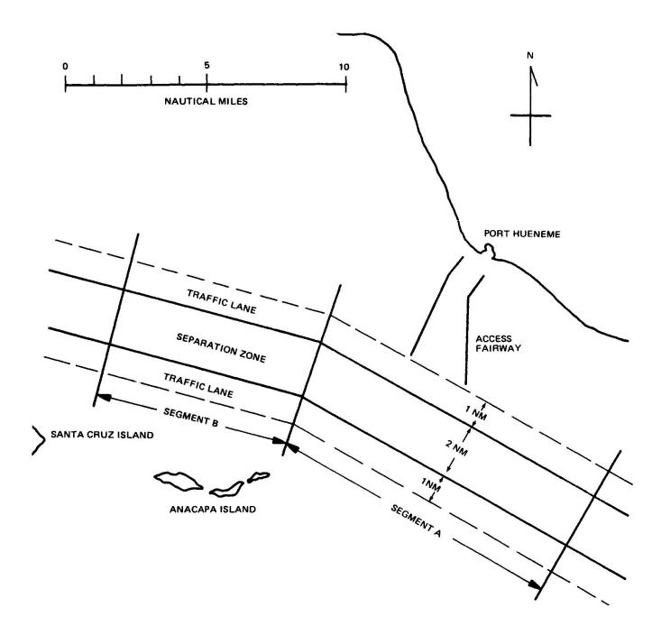
Figure 1. The Santa Barbara Channel Traffic Separation Scheme Showing Segments A and B Used to Develop Various Simulation Scenarios
