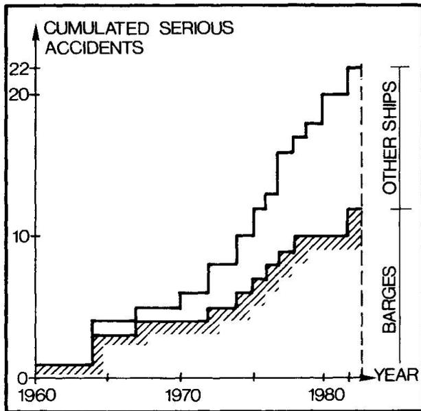
Fig. 1 Serious ship collisions with bridges 1960-1982.
