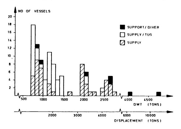
Fig 2. Supply vessels in the Veritas class - 1980.
