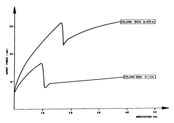
Fig. 7. Force/indentation curve for stern impact with infinitely stiff cyliner. Boat displacement 5000 t.
