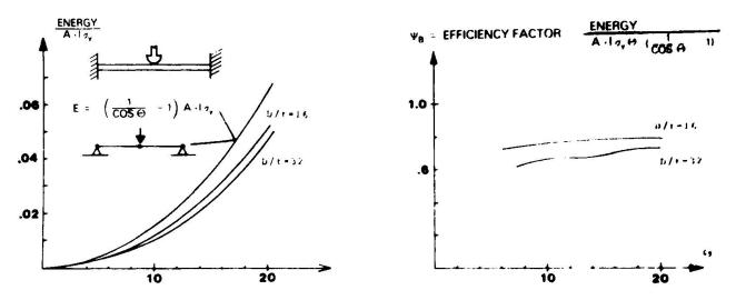
Fig. 12. Energy absorption in axially restrained members [29].
