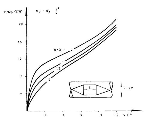
Fig. 10. Load indentation relation for steel tubes.
