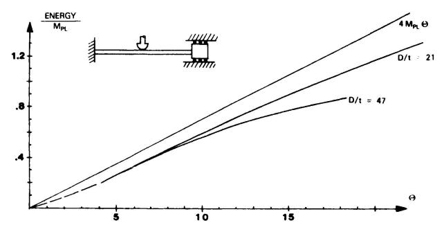
Fig. 11.- Plastic energy absorption in a three hinge mechanism.
