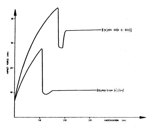
Fig. 5. Force/indentation curve for broadside impact with infinitely stiff cylinder. Boat displacement 5000 t.
