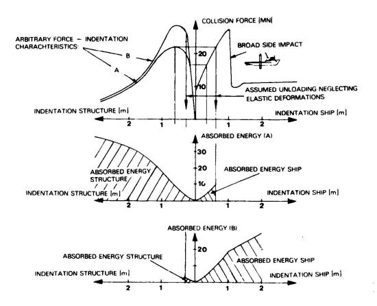
Fig. 3. Energy distribution ship/structure.
