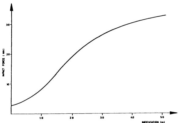
Fig. 6. Force/indentation curve for bow impact with infinitely stiff cylinder. Boat displacement 5000 t.
