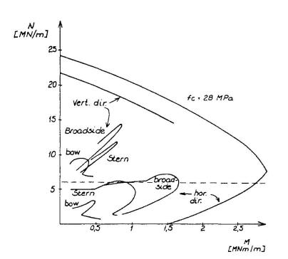
our case, punching will govern small areas only; thus the membrane effect is neglected and the transverse shear force is simply taken as the total load uniformly distributed over the perimeter. Locally, this average value may be slightly exceeded in certain cases; however, the ship side will bridge a possible concentrated failure.
