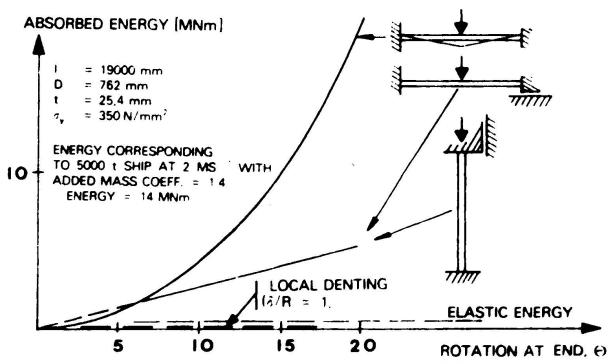
Fig. 13 Comparison of energy absorption capabilities [29].
