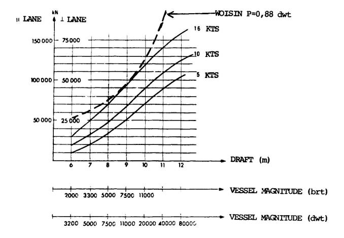
Fig. 1. Nordic Road Federation. Recommended impact force.
