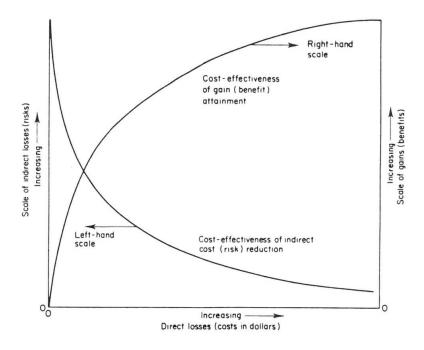
$\frac{\text{Fig. 4}}{(\text{cost})}$  Gain and indirect loss curves as a parametric function of direct loss expenditures.
