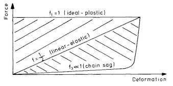
Fig.5 Possible work diagrams for converting collision energy
