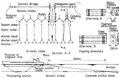
Fig.8 Protective system with elastic nylon ropes. From [8]
