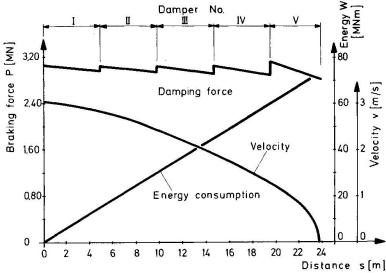
Fig.10 Force and speed diagram of the protective system for the Taranto Bridge. From /97
