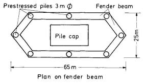
Fig.14 Protective system with vertical piles. From /87
