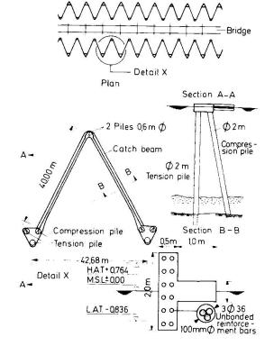
Fig.15 Protective system with tension piles. From [87
