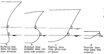
buoyancy of the arrestor device, the friction between arrestor device and ship, the shape of the arrestor device — a round member will more likely roll under the bow than an oval one—and the inclination of the ship's bow. Furthermore, a ship's bow often consists of a cast iron part which may be relatively sharp-edged and can cut the anchor cables with its submerged portion.
