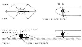
Most tests were performed with a 250,000 DWT and a 150,000 DWT tanker. Some were carried out with 50,000 DWT container Altogether approximately 500 tests were performed. The model length scales were 1:94 and Froude-scaling was applicable. The rubble mound slopes and islands of uniform consisted crushed stones, corresponding to 400 kg stones in nature. The slopes were in all tests 1:1.5 and the berms were horizontal.
