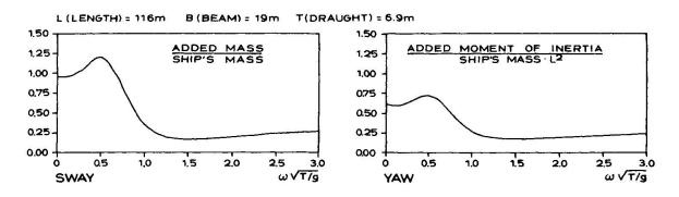
Fig. No. 1 Added Mass and Moment of Inertia for Sway and Yaw.
