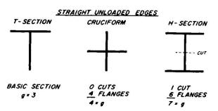
Fig. 2. Methods of cutting simple elements to determine "g". (From ref. [8]).
