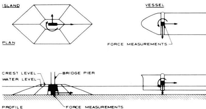
Most tests were performed with a 250,000 DWT and a 150,000 DWT tanker. Some were carried out with a 50,000 DWT container ship. Altogether approximately 500 tests were performed. The model length scales were 1:94 and 1:79. Froude-scaling was applicable. The rubble mound slopes and islands consisted of uniform sharply crushed stones, corresponding to 400 kg stones in nature. The slopes were in all tests 1:1.5 and the berms were horizontal.
