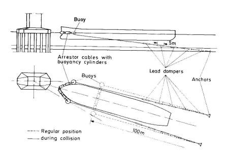
The ship's energy is absorbed for each anchor chain by 5 dampers connected one behind the other, each 5m long. The dampers consist of a steel pipe, in which a drawbar absorbs energy through the deformation of a lead filling. The work lines of the dampers were determined by full-size model testing.
