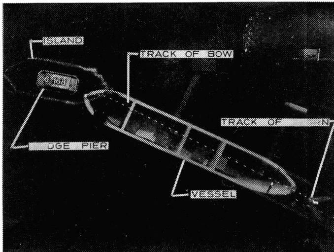
The tracks of the vessels were registered by a camera which was mounted above the protection structure. Flashing lights on the bow and the stern clearly indicated the tracks and the velocities of these parts of the vessel, see Fig. No. 5.
