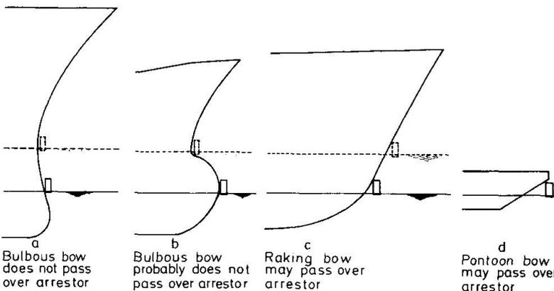
Fig.13 Typical bow shapes and floating systems. From [8]
