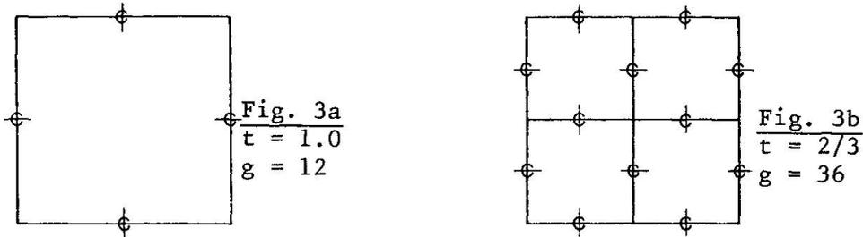
Figures 3a and 3b have the same outside dimensions. Cuts are made so as to produce simple flanged elements. The total cross sectional area  $A$  is the same for 3a and 3b when  $t = 1$  in Fig. 3a and  $t = 2/3$  in Fig. 3b. The application of Gerard's relationship shows that 3b has a crippling strength and a resistance to failure 27.6% greater than 3a; conversely, for the same crippling strength, 3b will be lighter than 3a.
