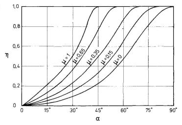
η = absorbed collision energy initial ship's energy
