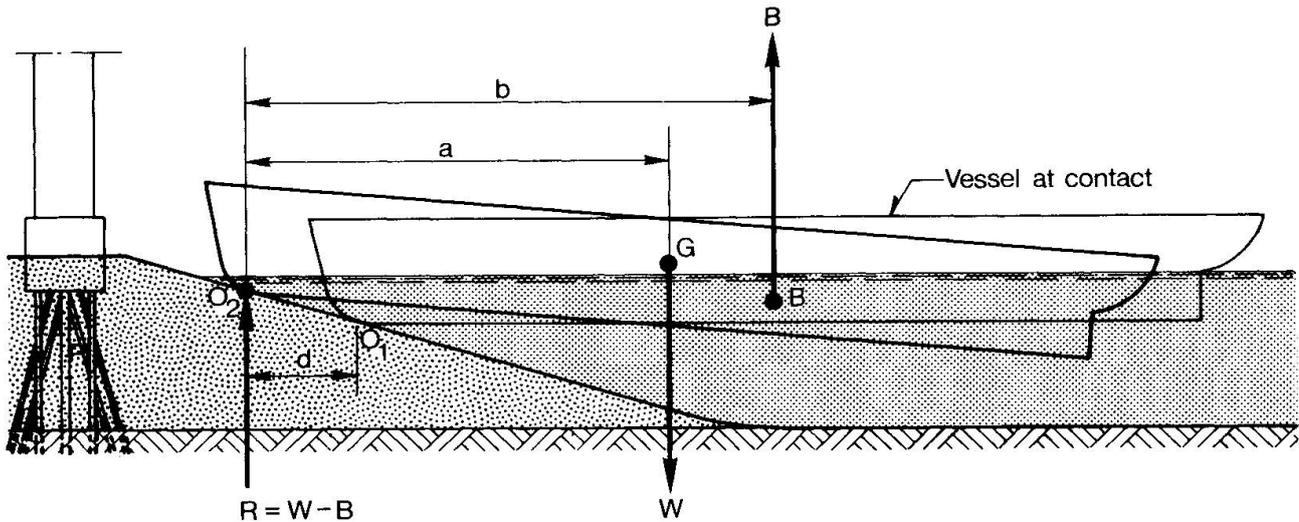
Fig. 6. Weight-buoyancy equations for ship meeting artificial island.
