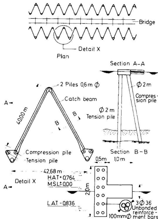
Fig.15 Protective system with tension piles. From [8]
