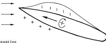
Fig. 5. Turning moment due to negative pressure field caused by current on hull.
