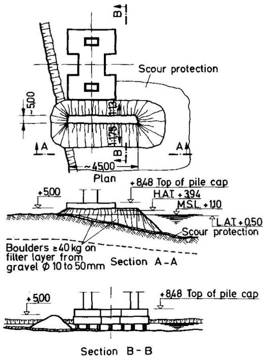
The width of its crown was determined on the basis of the model tests for the Great Belt Bridge.
