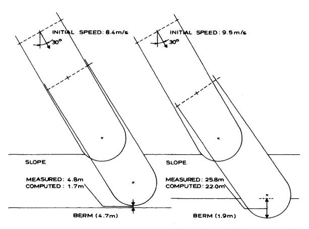
Fig.No. 10 Measured and Computed Penetrations for an Obliquely Incoming 250,000 DWT Tanker, Draught 10 m.
