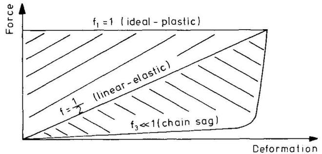
Fig.5 Possible work diagrams for converting collision energy
