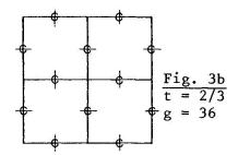
Figures 3a and 3b have the same outside dimensions. Cuts are made so as to produce simple flanged elements. The total cross sectional area A is the same for 3a and 3b when t=1 in Fig. 3a and t=2/3 in Fig. 3b. The application of Gerard's relationship shows that 3b has a crippling strength and a resistance to failure 27.6% greater than 3a; conversely, for the same crippling strength, 3b will be lighter than 3a.
