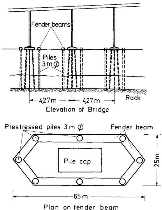
Fig.14 Protective system with vertical piles. From [8]
