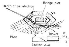
Fig.19 Operation of protective islands from model tests. From [227]
