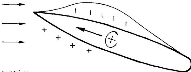
Fig. 5. Turning moment due to negative pressure field caused by current on hull.
