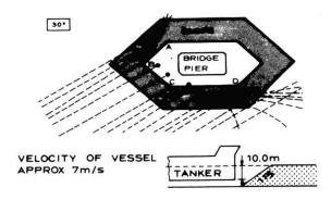
Fig. No. 12 shows that the important deflective characteristics are maintained for vessels approaching under a more infavourable approach angle.
