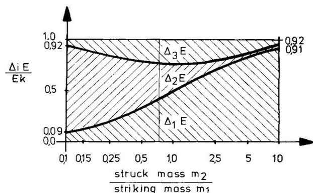
Fig.12 Distribution of the collision energy between anchored protective ship and colliding ship according to Woisin
