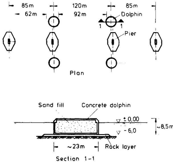
Fig. 16 Sliding caissons. From [17]
