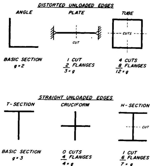
Fig. 2. Methods of cutting simple elements to determine "g".
