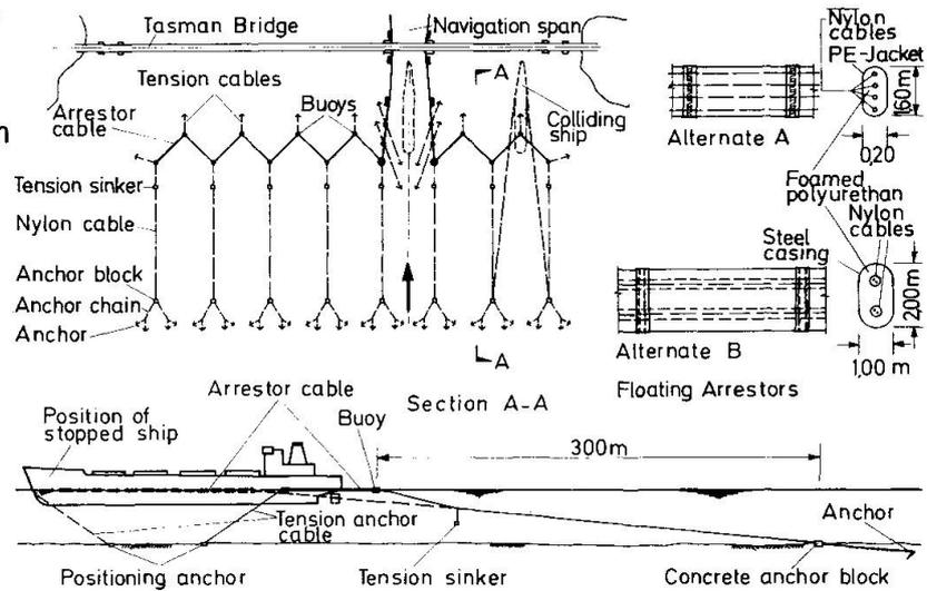
Fig.8 Protective system with elastic nylon ropes. From [8]
