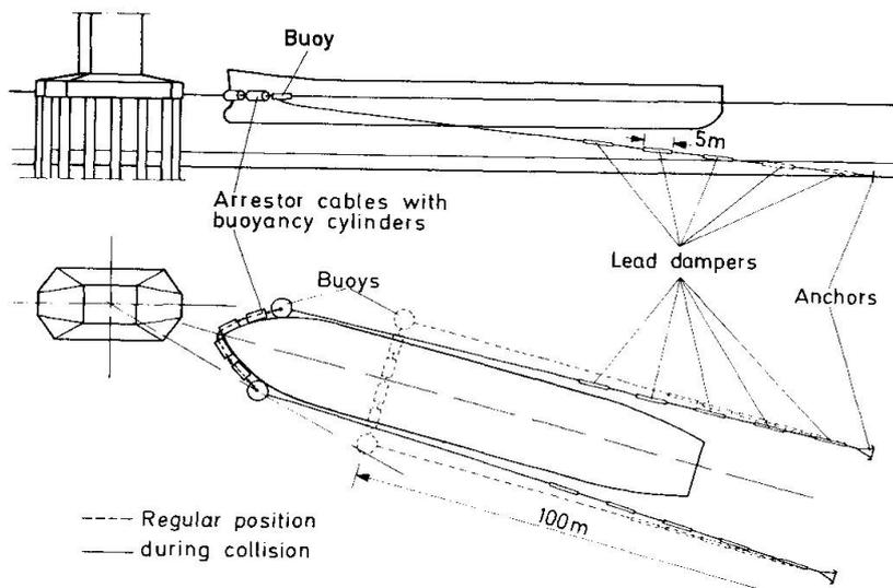
The ship's energy is absorbed for each anchor chain by 5 dampers connected one behind the other, each 5m long. The dampers consist of a steel pipe, in which a drawbar absorbs energy through the deformation of a lead filling. The work lines of the dampers were determined by full-size model testing.
