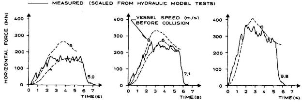
Fig. No. 9 Computed and Measured Collision Forces for a 250.000 DWT Tanker, Draught 10 m. Berm Level 1.9 m (MWL).
