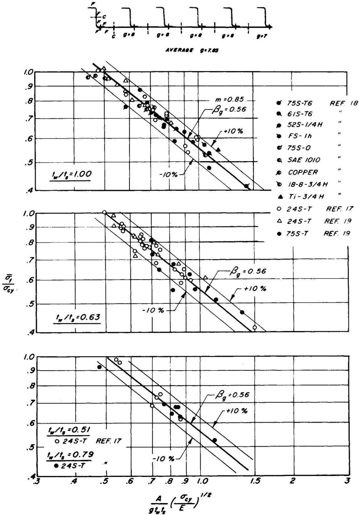
Fig. 1. Crippling data on Z-stiffened panels.
