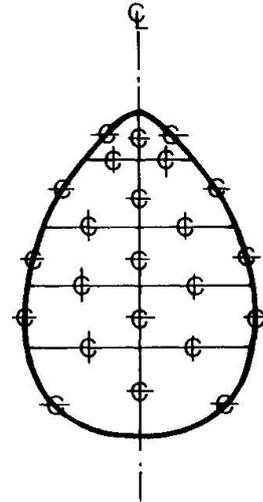
Fig. A-3. Section at frames 157½ - 158.
