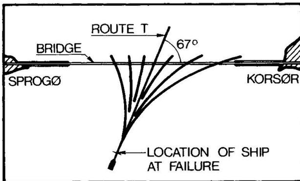
In the Great Belt Bridge project [8] and [9], a distribution of courses of ships out of control, as shown in fig. 8, was assumed. All courses within a chosen curvature range were regarded as equally frequent. The idea was to represent, in a simple way, an average of possible movements of the most important part of the local shipping.
