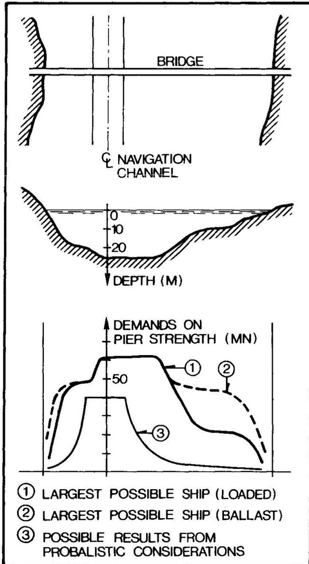
For major bridges it is thus reasonable to treat the problem of ship collision by means of a probabilistic approach, since this allows us to weigh the risk level against the construction cost on a rational basis.
