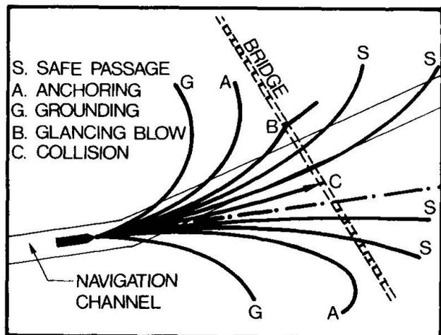
Some of these uncontrolled vessels will pass the bridge safely, and others will stop or go aground, but a tiny fraction will hit one of the piers or the superstructure of the bridge, depending on the location of the piers and the vertical clearance.
