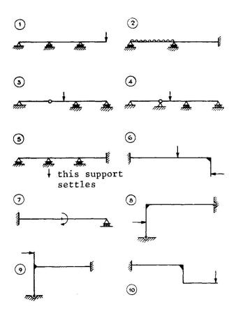
Fig. 1: Part of test paper devised by Brohn and Cowan [7]
