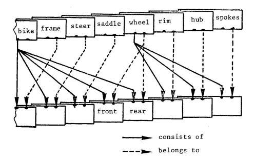
Fig. 5. Occurance diagram of bicycle assembly.
