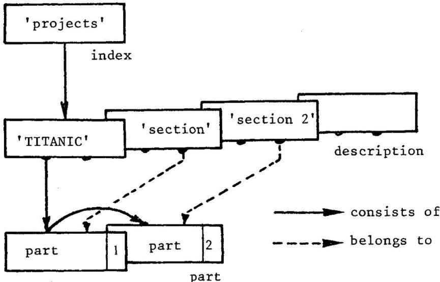
Fig. 17. Ship divided into sections.
