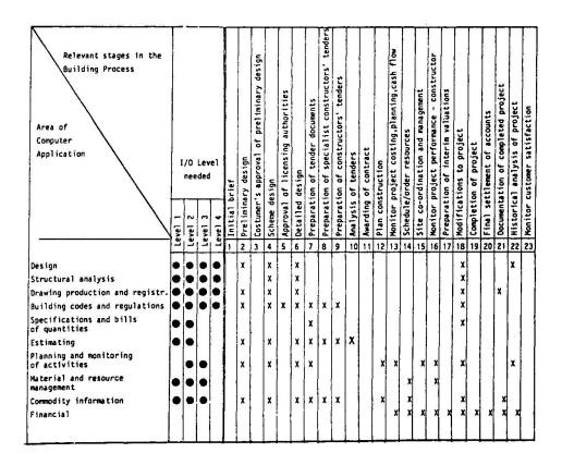
Figure 1 Areas of Computer Application v. Stages in the Building Process with 1/0 levels
