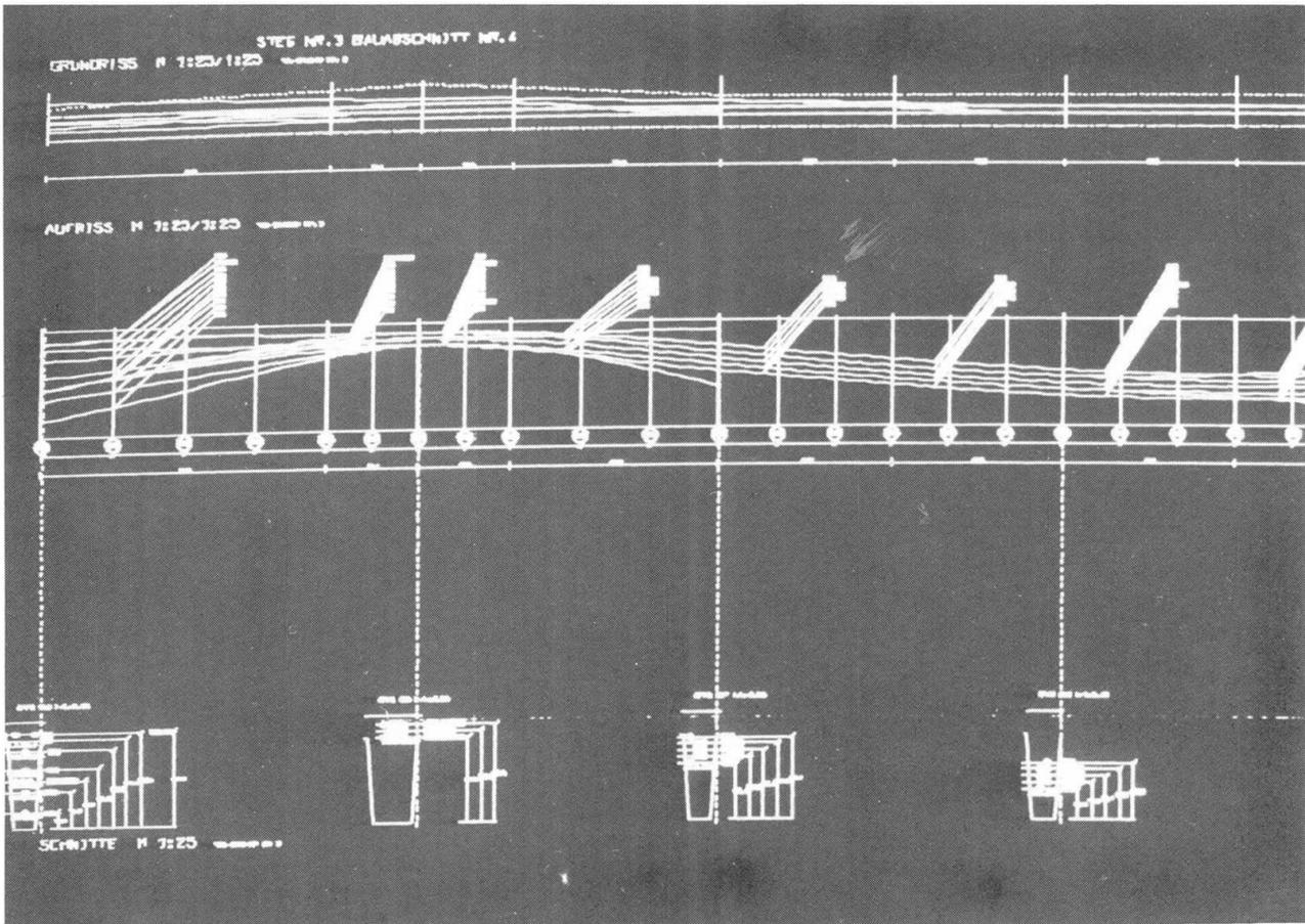
Fig. 2 Example of pre-stressing cable plan
