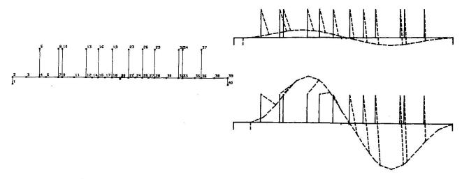
Fig. 3 Idealization of an arch by means of a fictitious straight beam and typical deformed shapes.
