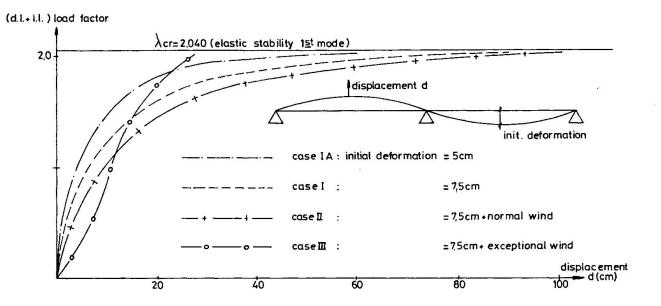
Fig. 4 Load factor versus out-of-plane displacement curves under different step-by-step loadings.
