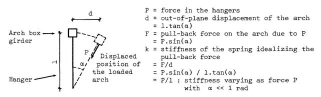
Figure 2 Pull-back forces of the hangers
