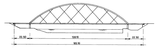
Figure 1 Side view and cross section of the bridge
