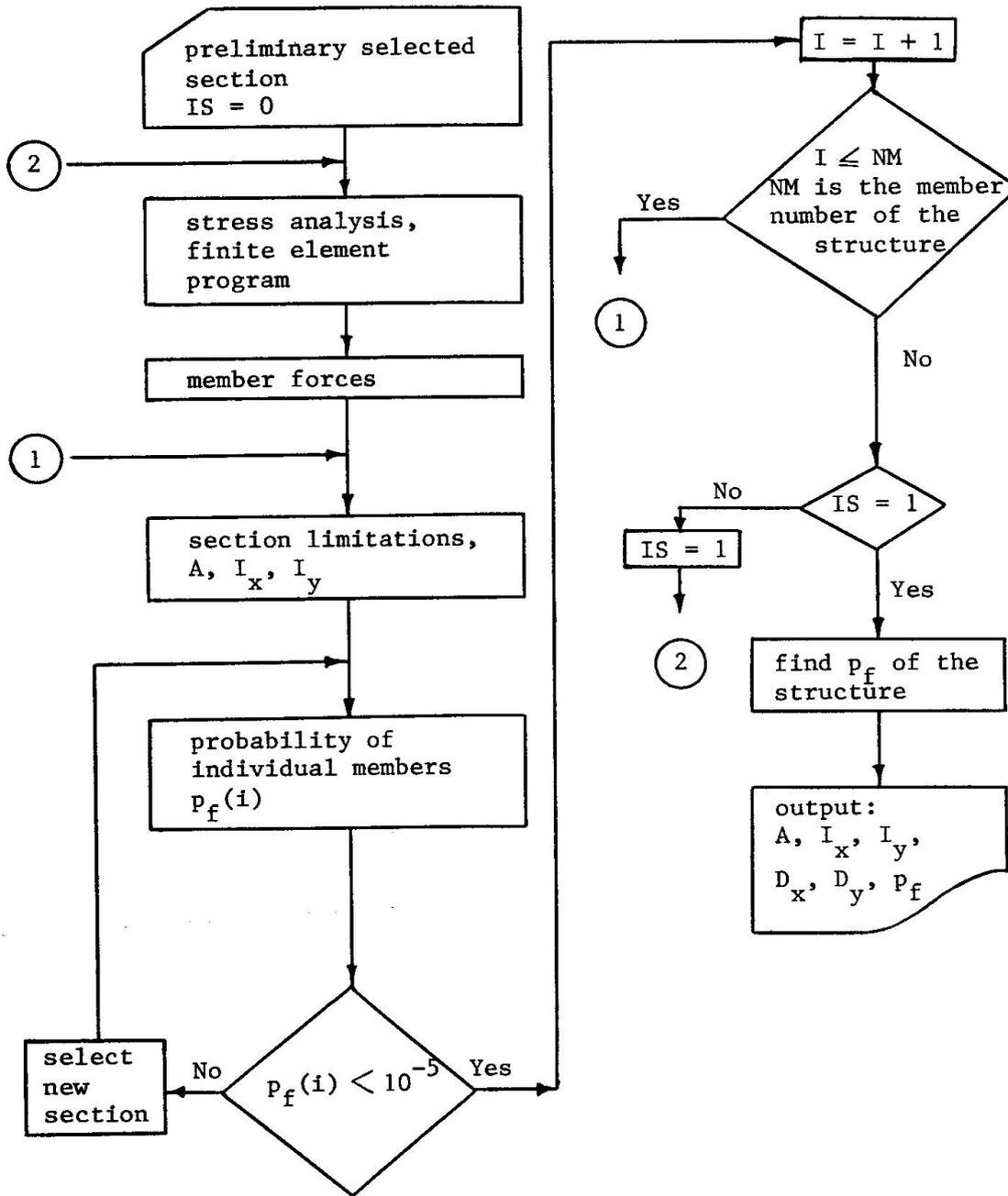
Fig. 6 Flow Chart of the Program for Optimum Design to Select Proper Sections
