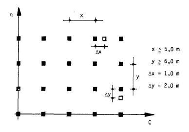
Fig. 6: Structural grid of the ground floor
