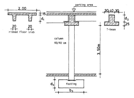
Fig. 5: Details of the supermarket building's structure
