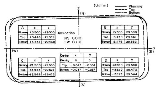
Fig. 5 Error of setting-caisson
