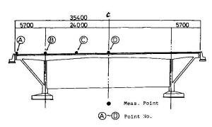
Fig. 3 An over-bridge for load capacity and vibration tests.
