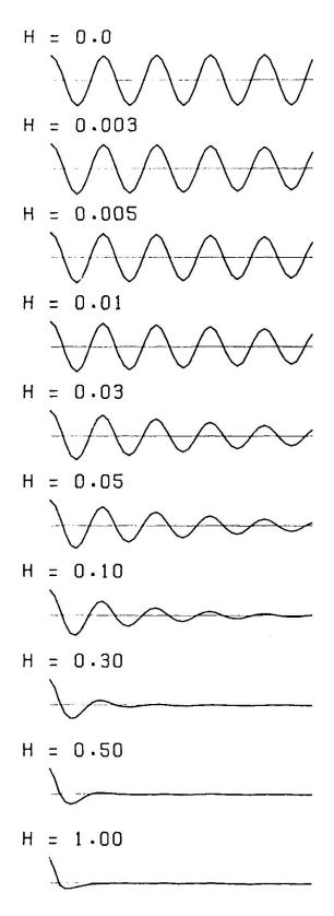
Fig.ll Response of a simple pendulum with a dashpot.
