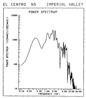
SAMPLING TIME = 0.020 SEC SAMPLE DATA = 1024 SMOOTHED SPECTRA BY HAMMING WINDOW 5 CYCLES START COUNTER NUMBER = 1
