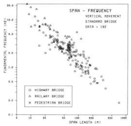
Fig.1 Relationship of fundamental frequency to span.
