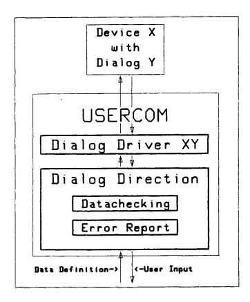
Fig. 3: Structure of the USERCOM
