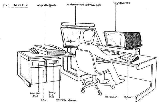
Fig 6 Sample workstation layout for Level 2
