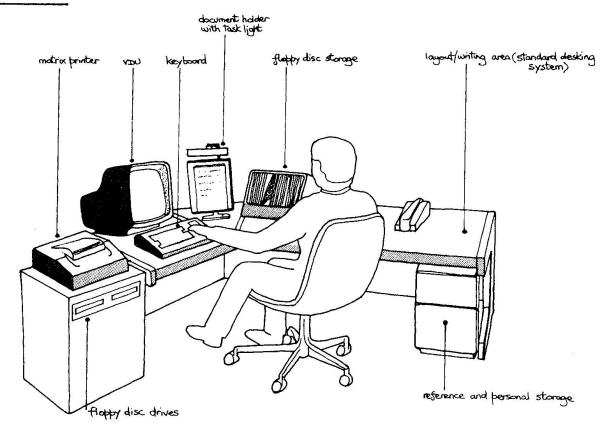
Fig 7 Sample workstation layout for Level 1
