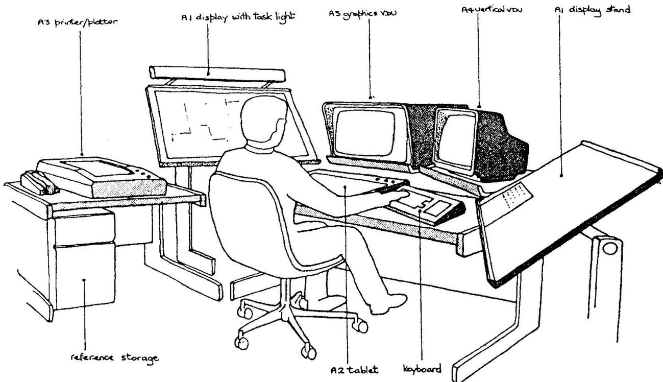
Fig 5 Sample workstation layout for Level 3
