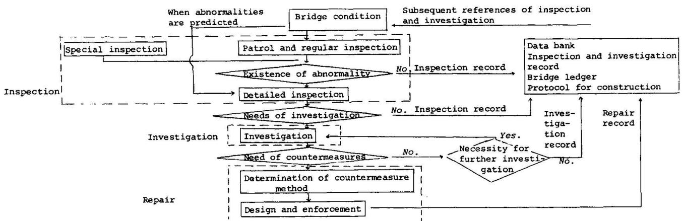
Figure 1. Flow diagram of inspection, investigation and repair works
