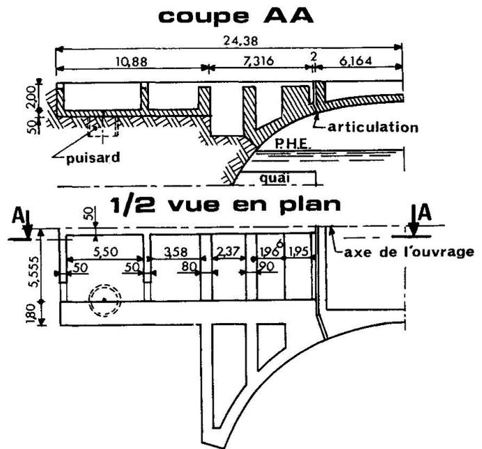
Fig. 5 : Abutment drawing.
