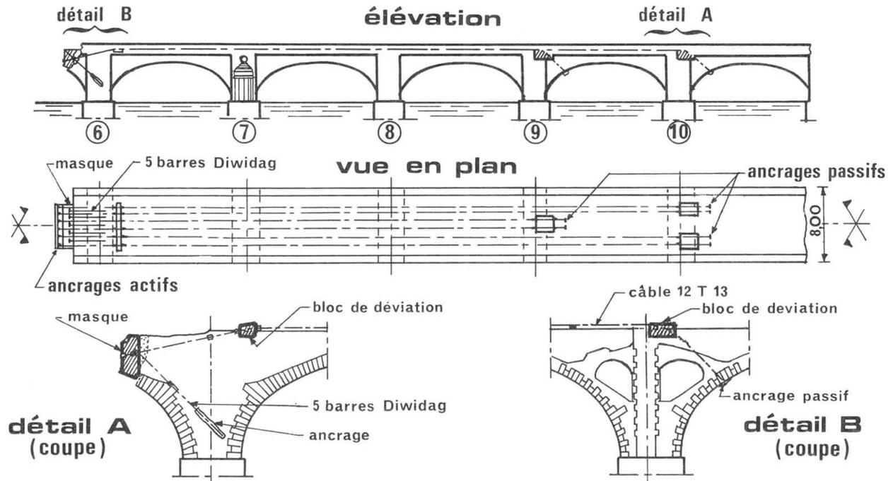
Fig. 2 : Pier 6 : temporary prestressing.
