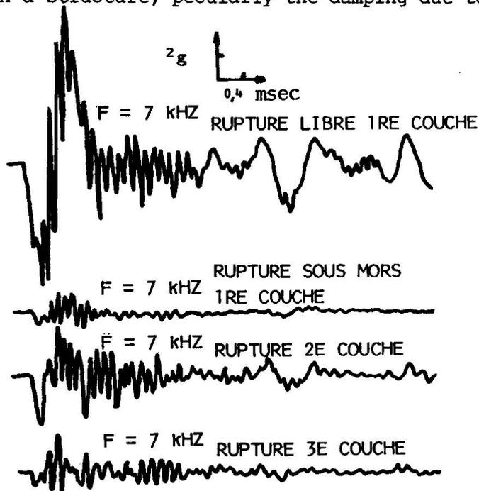
FIGURE N° 1 - Recording of the first wave in various cases of individual wire fracture in a cable, at 21 m far from the breaking point
