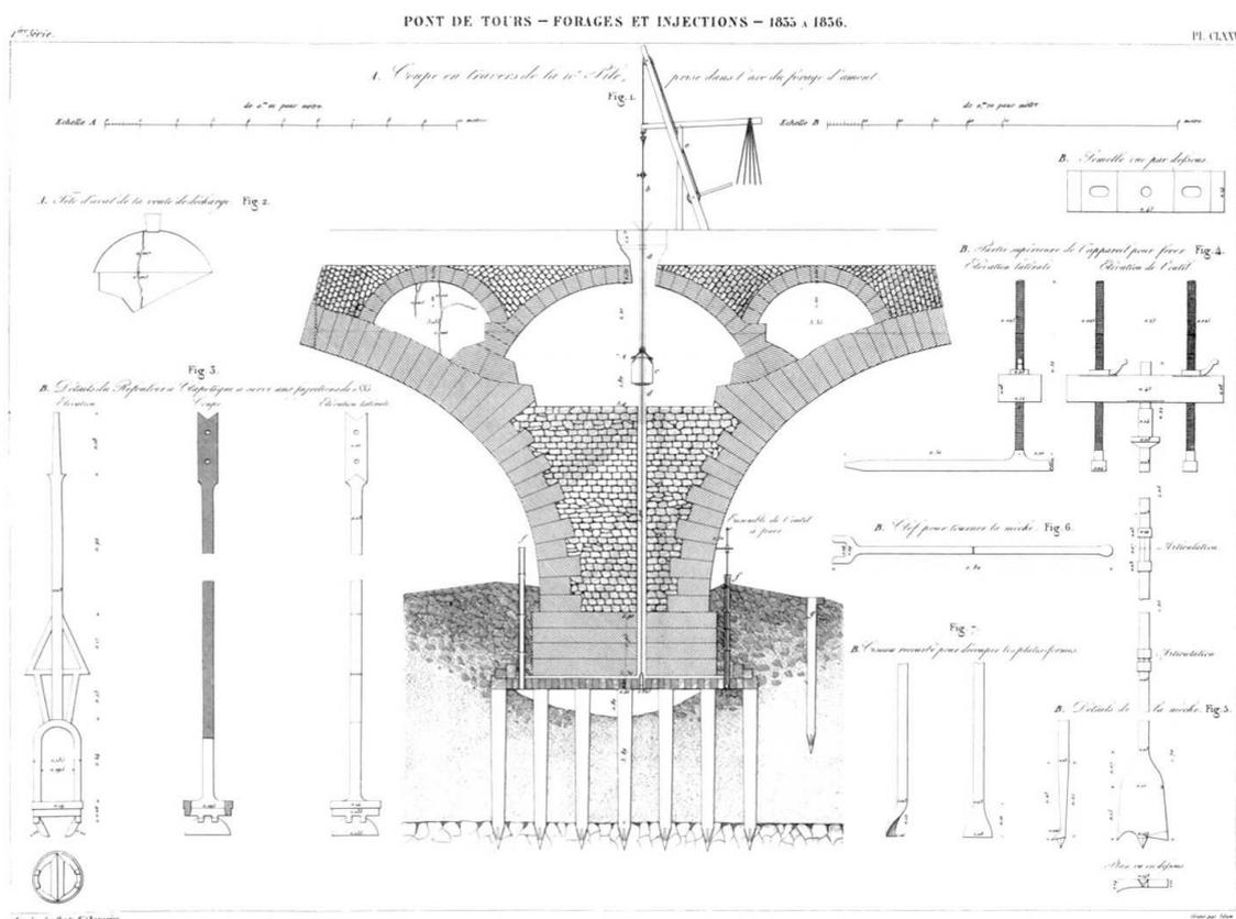
Fig. 1 : 1835 – Lime injections.
