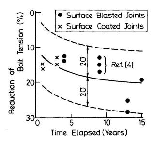
Fig. 3 Aging in Bolt Tensions
