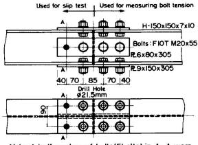
Note: A half number of bolts(5bolts) in A-A were loosened before slip tests.
