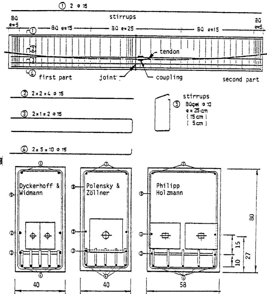
Fig.3 Reinforcement of the test beams and cross-sections
