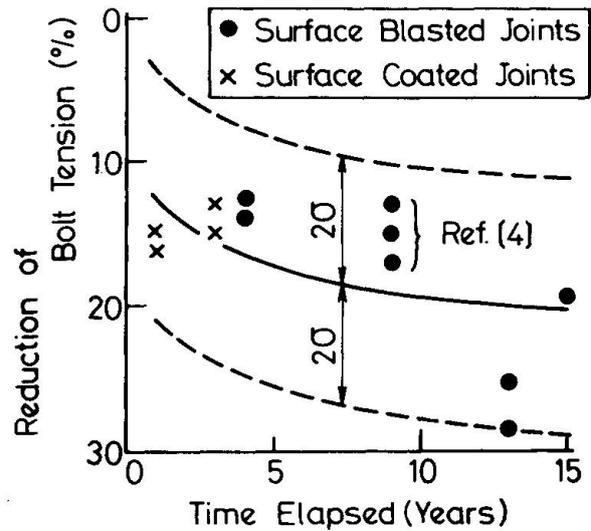
Fig. 3 Aging in Bolt Tensions
