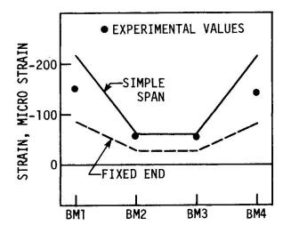
Fig. 3. Midspan, bottom flange strains resulting from post-tentioning: Bridge #1.
