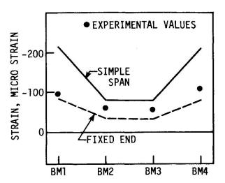
Fig. 4. Midspan, bottom flange strains resulting from post-tentioning: Bridge #2.
