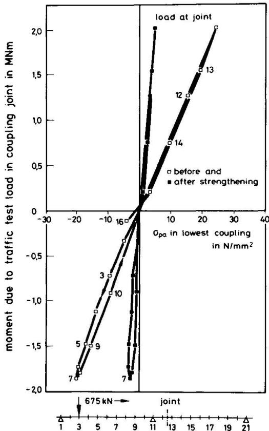
Fig. 6 Stress amplitude of prestressing steel of the lowest coupling, depending on test load moment
