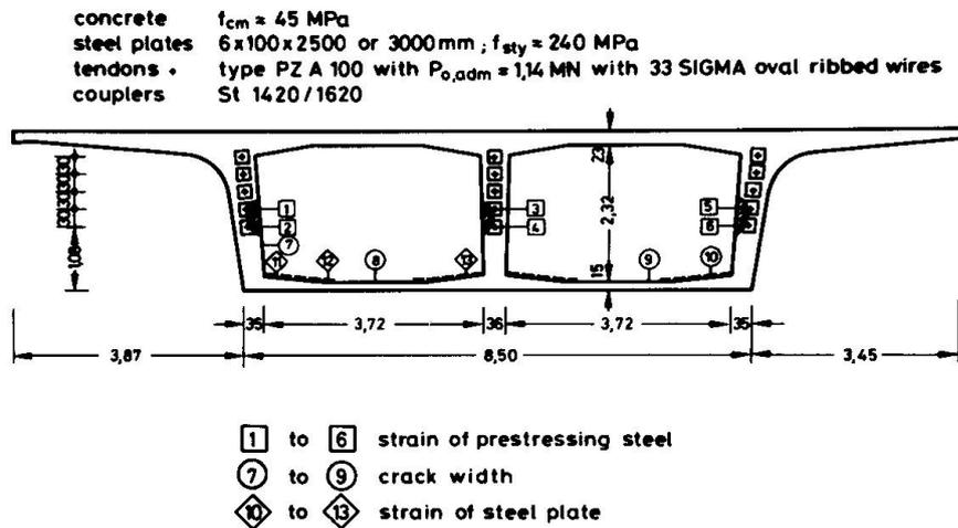
Fig. 5 Cross-section of bridge and other data
