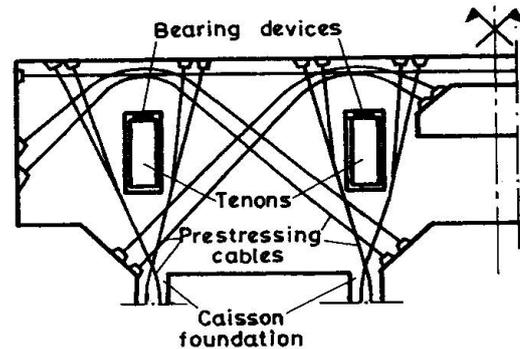
Fig. 4 - Abutment device
