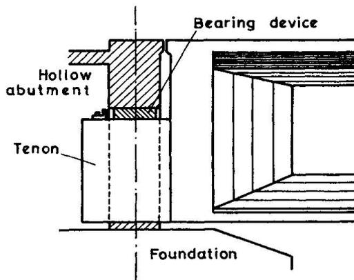
Fig. 3 - Abutment device
