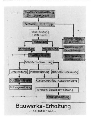
Fig. 9 shows how the supervision of structures is organized within our highway administration, taking the main inspection as an example. The main inspection is generally carried out by special inspection parties. Depending on the kind and the significance of the defects detected, the test results will set off different activities, which range from minor maintenance measures by the responsible road or motorway maintenance depot to the immediate closure of the bridge.
