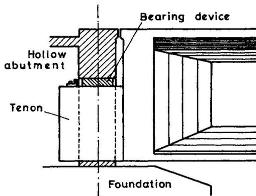
Fig. 3 - Abutment device
