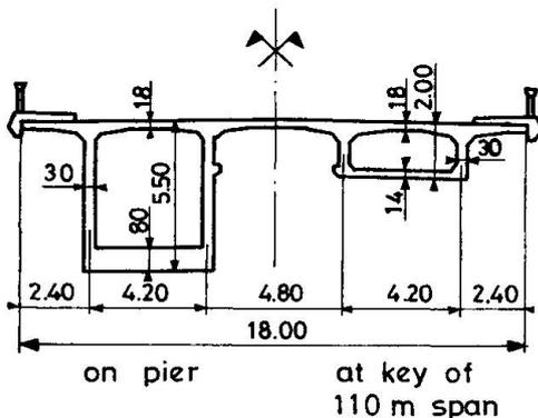
Fig. 2 - Cross-section
