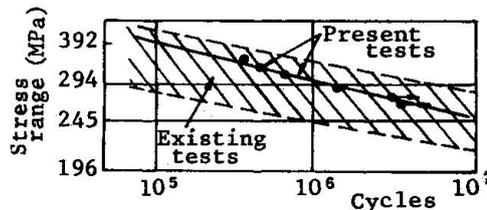
Fig.3 S-N relations of fillet weld of flange.
