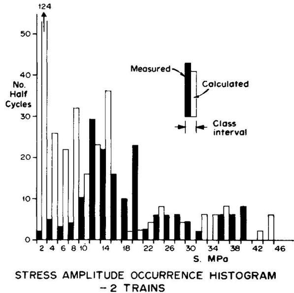
Fig. 7 Stress Amplitudes by Rainflow Method.
