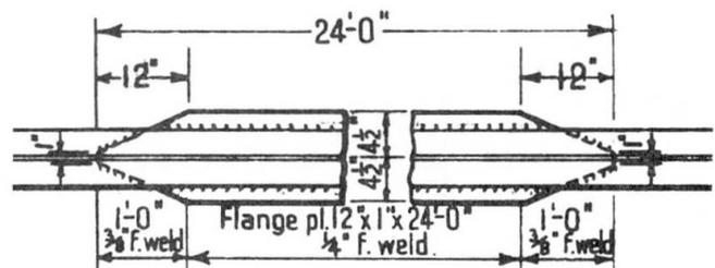
Fig. 2 Detail of Coverplate (from the original drawing).
