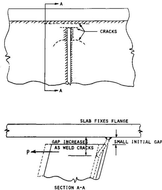
Fig. 3 Schematic of Crack Development
