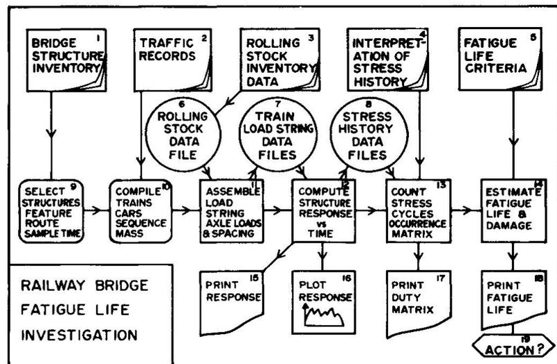
Fig. 4 Bridge Fatigue Life Flow Chart.
