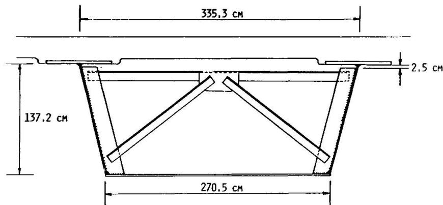
Fig. 1 Cross-Section of Curved Box Girder
