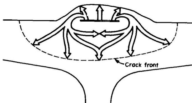
Fig. 9 Key to Crack Growth of Fig. 8.
