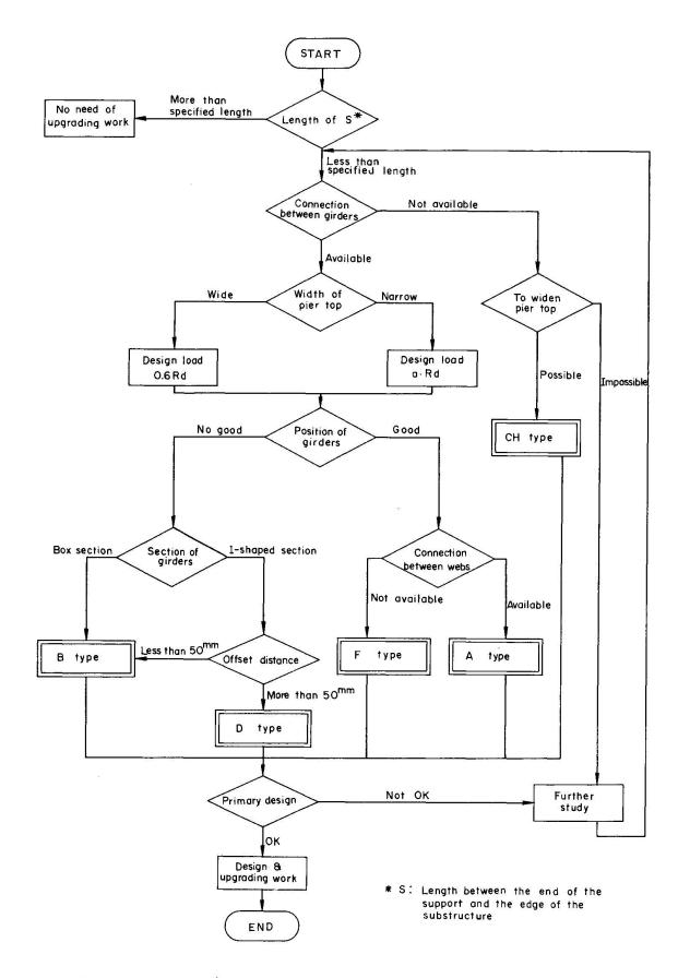
Fig 9 Procedural flow diagram on installation of fall-proof devices
