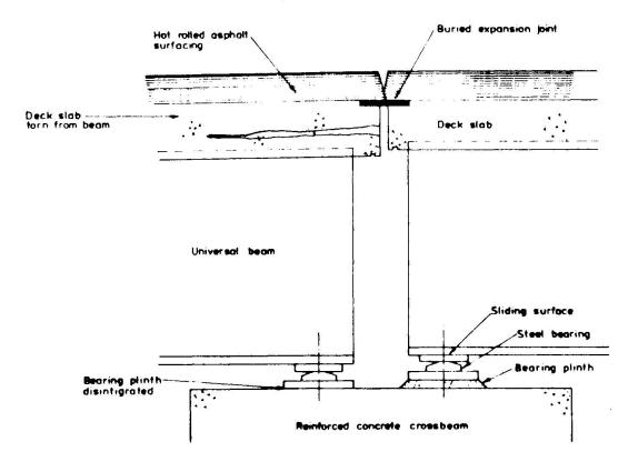
Fig. 1a Midland Links Viaduct - Detail of Bridge Bearings
