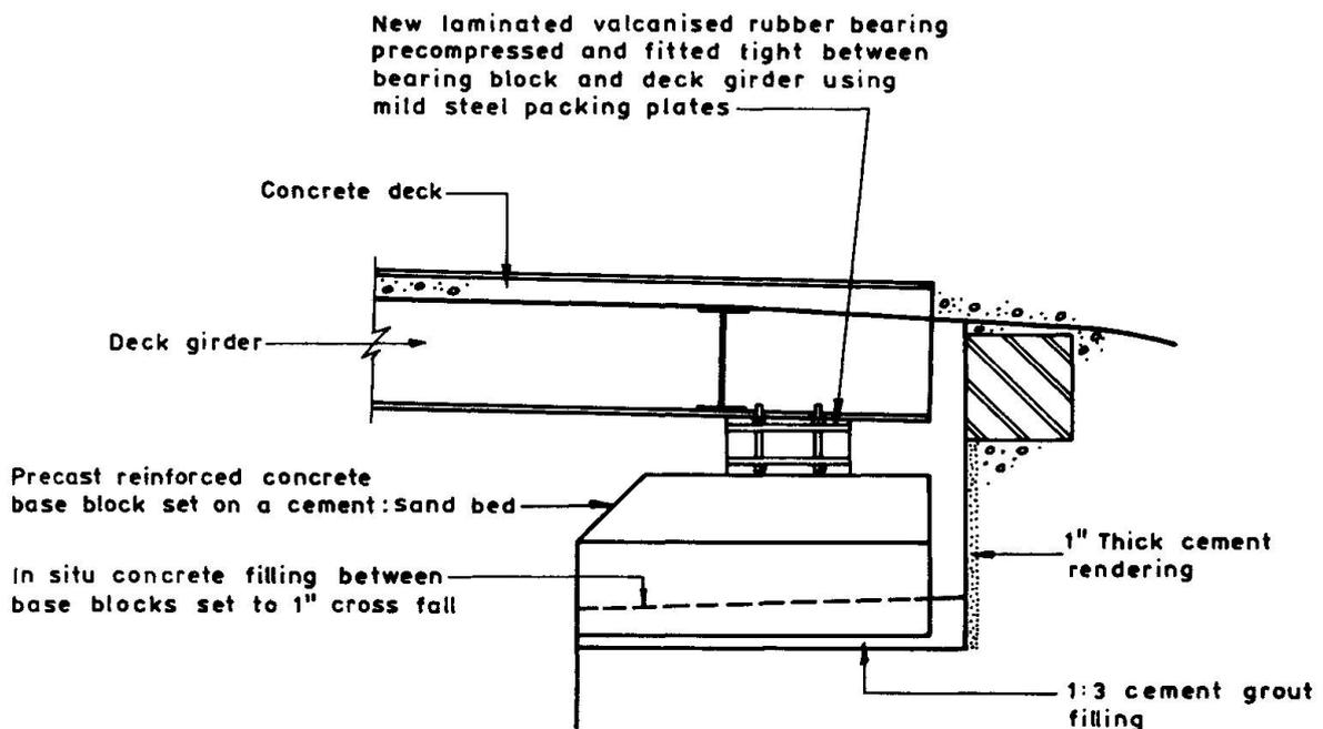
Fig. 2b Vauxhall Bridge - New Bearing in Position
