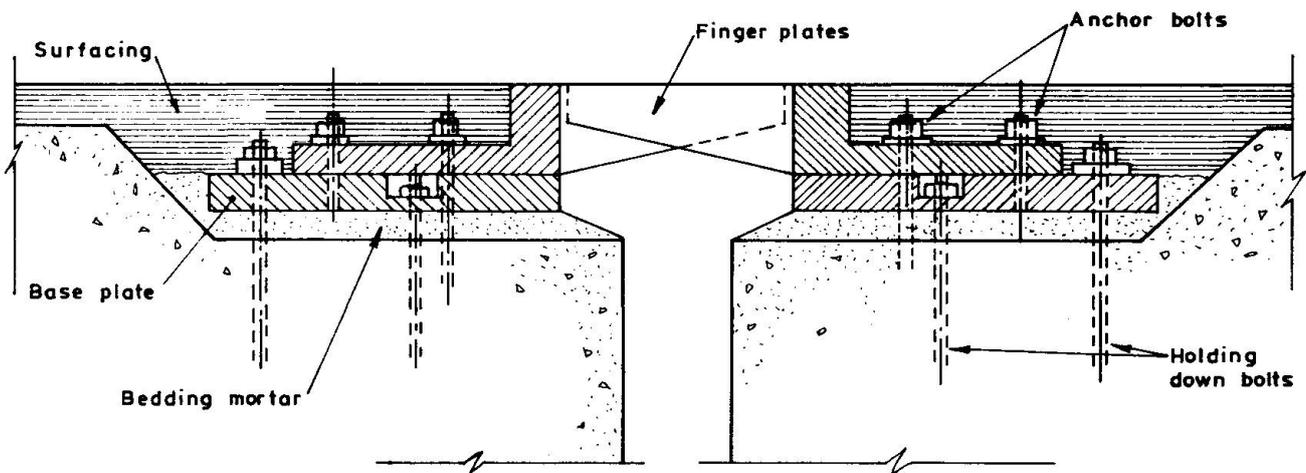
Fig. 10 Cantilever Joint
