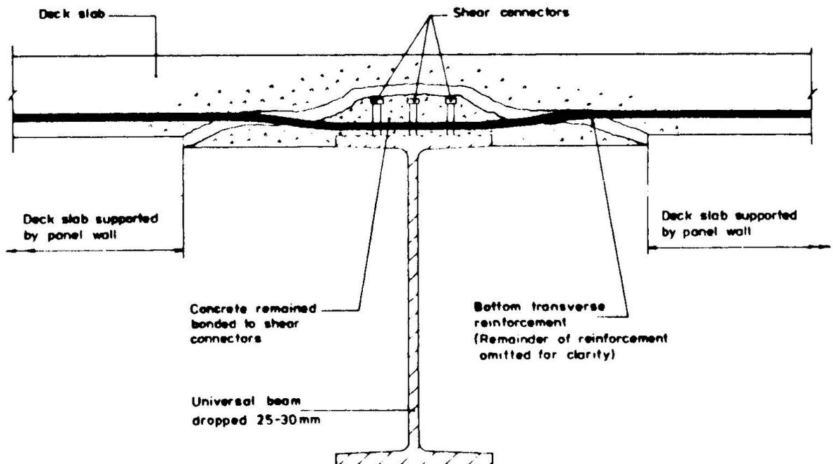
Fig. 1b Midland Links Viaduct - Typical Cracking in Deck Slab over Beams
