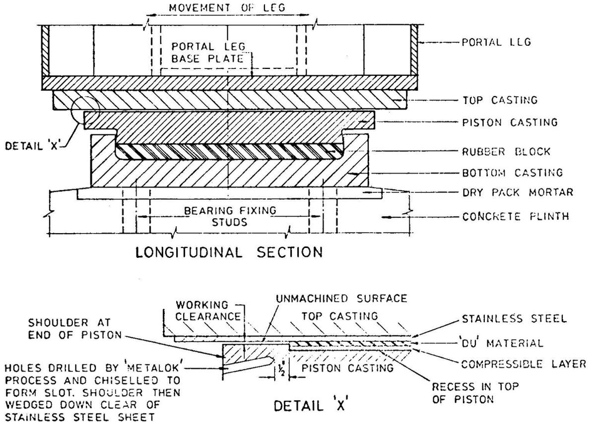
Fig. 4 Westway Section 6 - Details of Bearings
