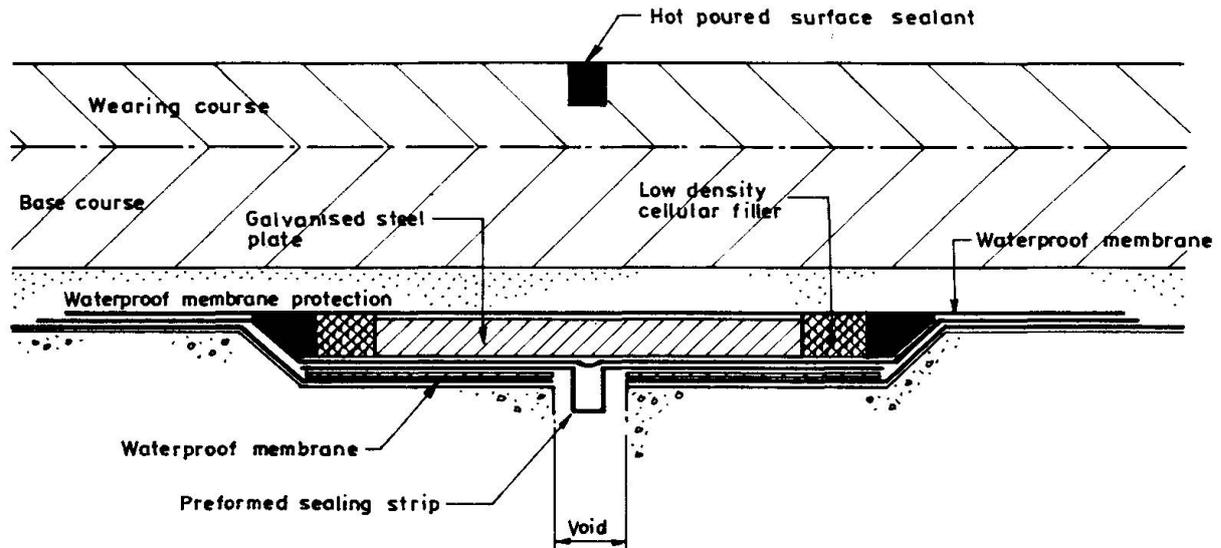
Fig. 7 Buried Deck Expansion Joint for Movements  $\pm 10$
