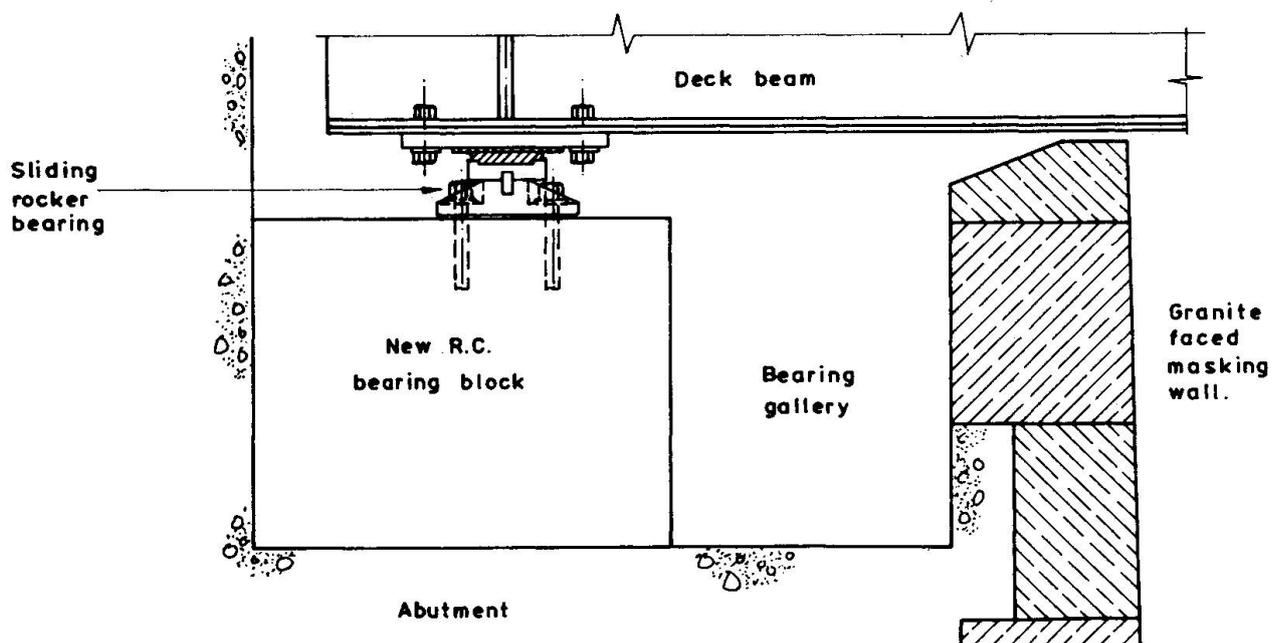
Fig. 3b Wandsworth Bridge - New Bearing in Position
