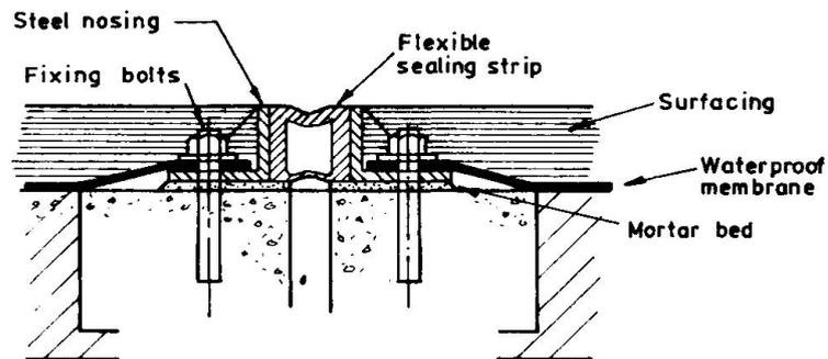
Fig. 8 Typical Expansion Joint for 20 - 50 mm Movement
