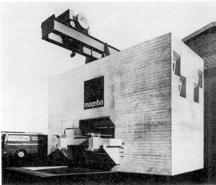
Fig. 18 Test Rig for Loads up to 100'000 kN
