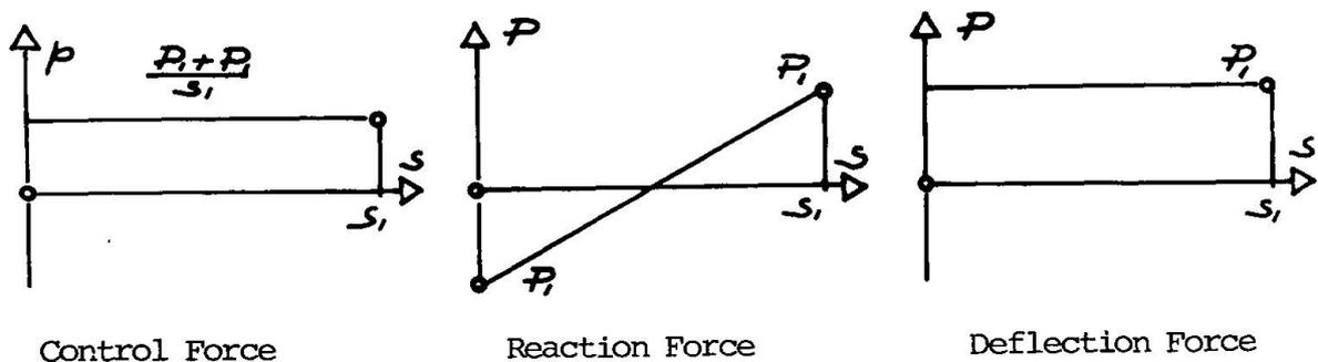
Fig. 17 Correlations of a Resilient Dual Control System
