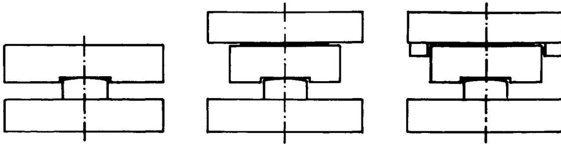
Fig. 3 Steel rocker bearing - fixed, multidirectional and unidirectional
