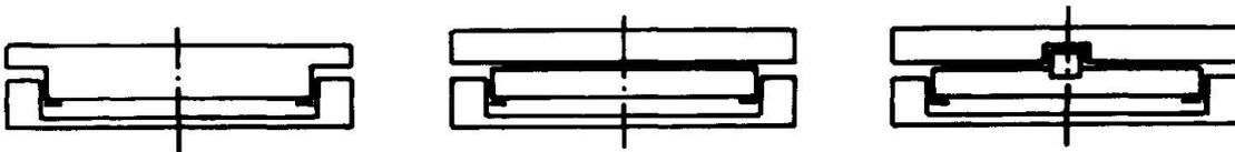
Fig. 5 Pot-type Bearing - fixed, multidirectional and unidirectional
