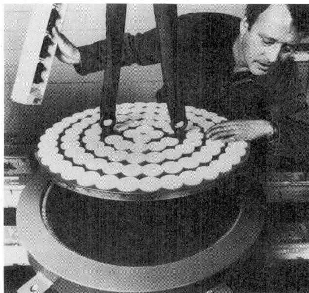
Fig. 9 Assembly of a Sliding Pot Bearing
