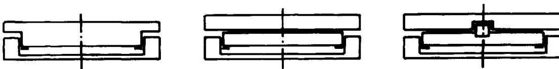
Fig. 5 Pot-type Bearing - fixed, multidirectional and unidirectional
