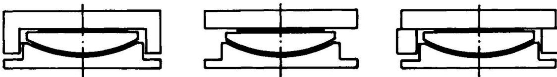
Fig. 4 Spherical Bearing - fixed, multidirectional and unidirectional
