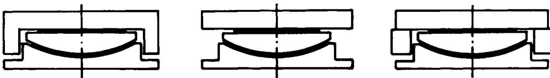
Fig. 4 Spherical Bearing - fixed, multidirectional and unidirectional
