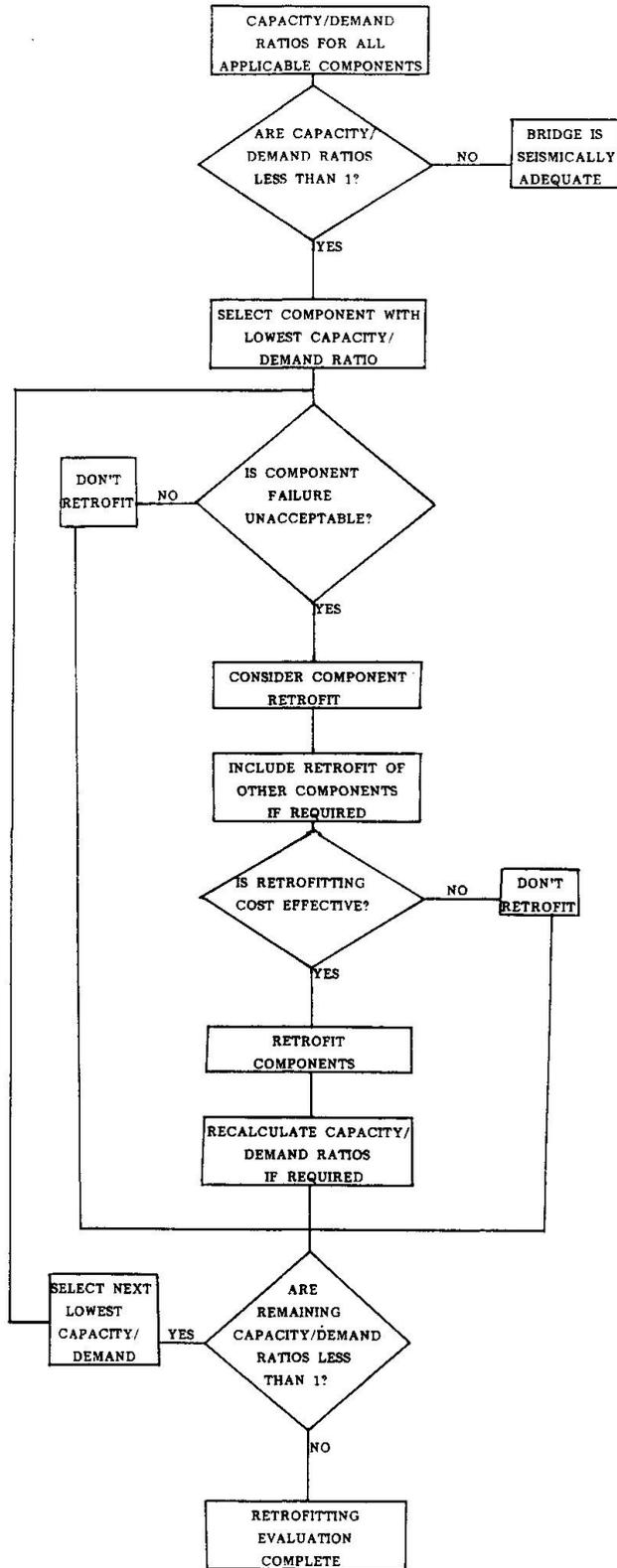
Fig. 3 Procedure for selecting retrofit methods
