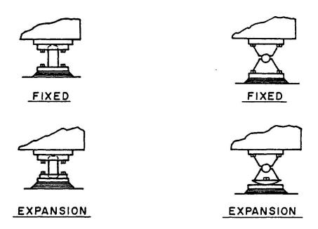
Fig. 6 Seismically vulnerable bridge bearings
