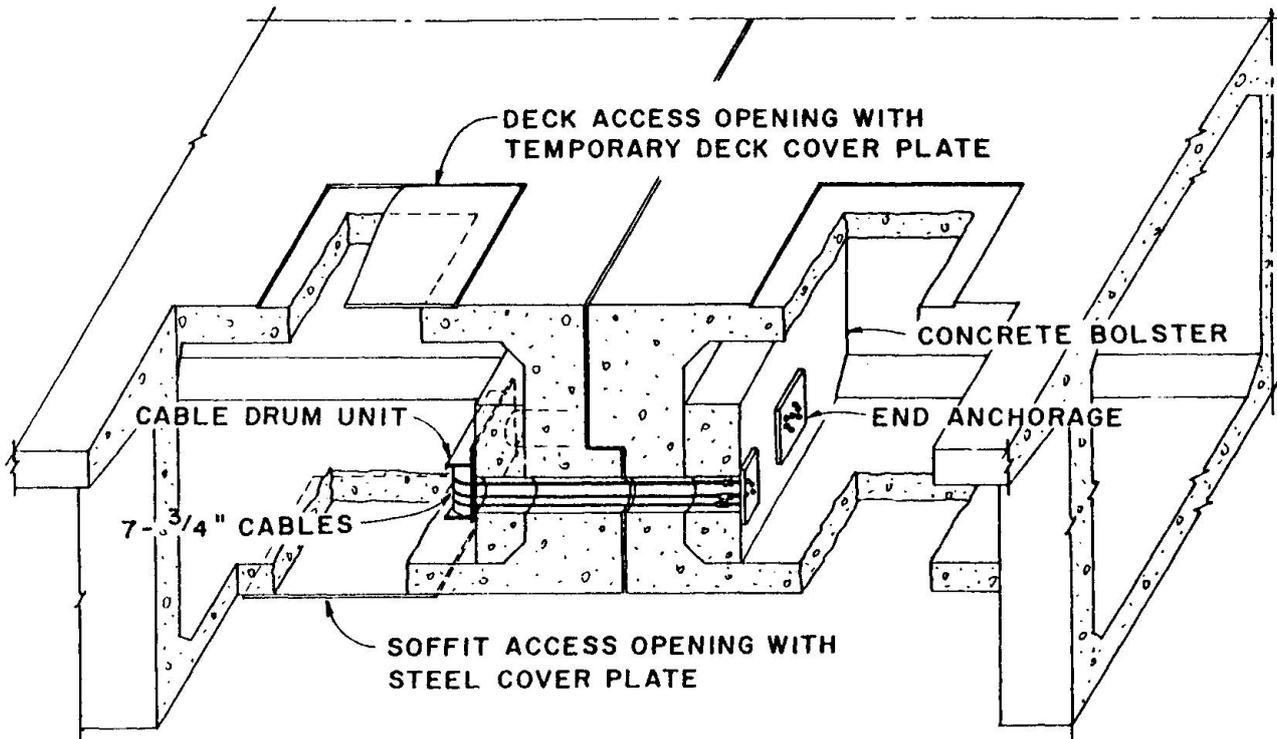
Fig. 5 Longitudinal joint restrainer for concrete box girder
