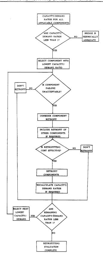
Fig. 3 Procedure for selecting retrofit methods
