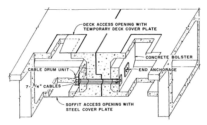
Fig. 5 Longitudinal joint restrainer for concrete box girder
