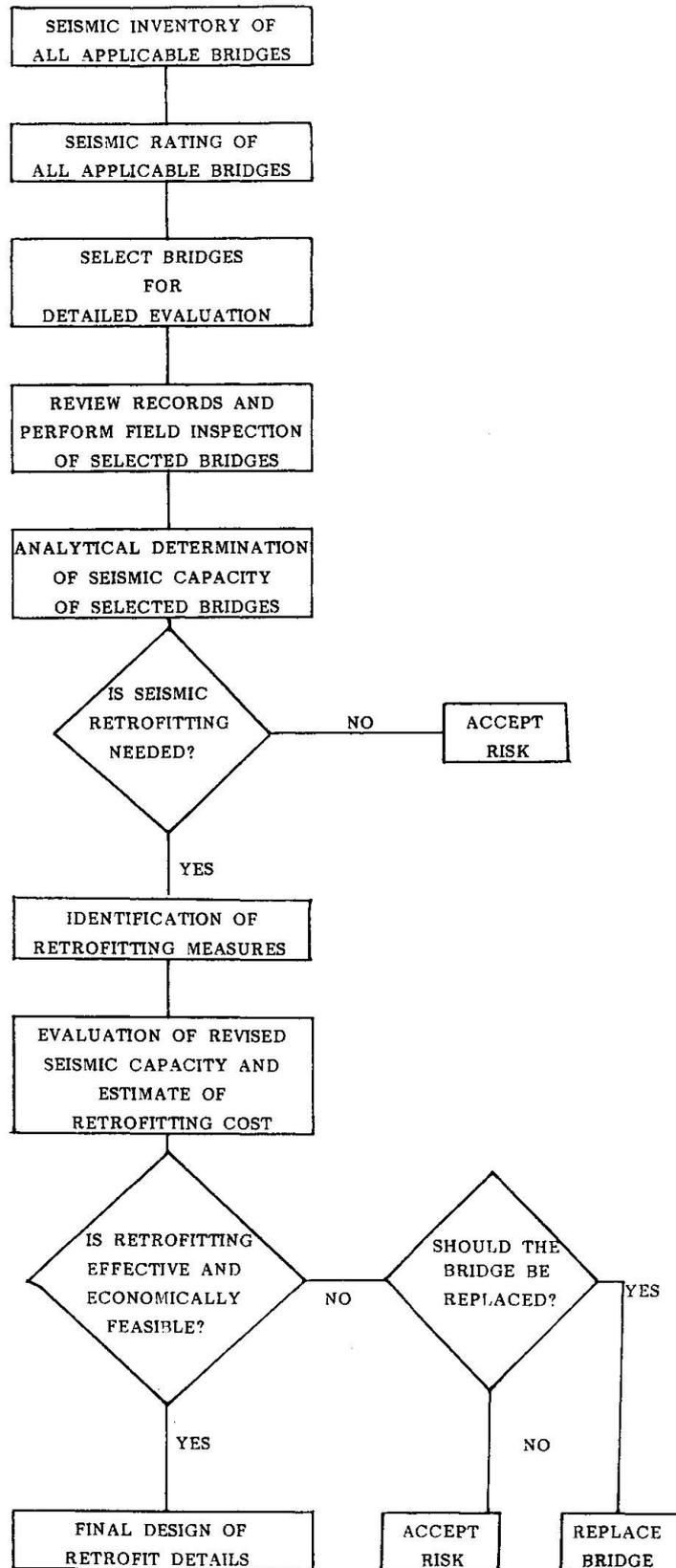
Fig. 2 Seismic retrofitting process for bridges
