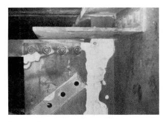
Figure 15 Crack at sharp notch
