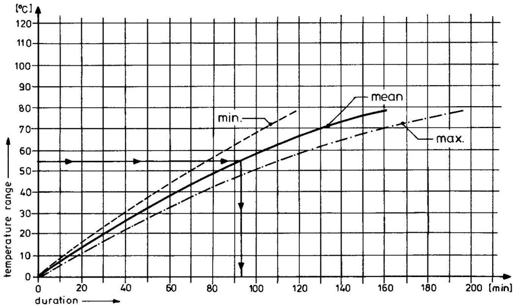
Fig. 6 Duration of Temperature Ranges for Paint Systems
