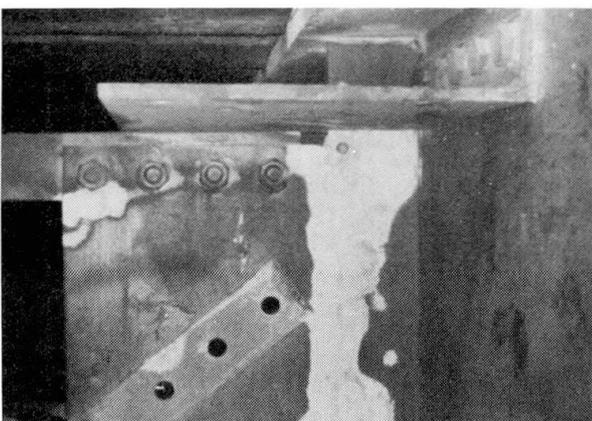
Figure 15 Crack at sharp notch
