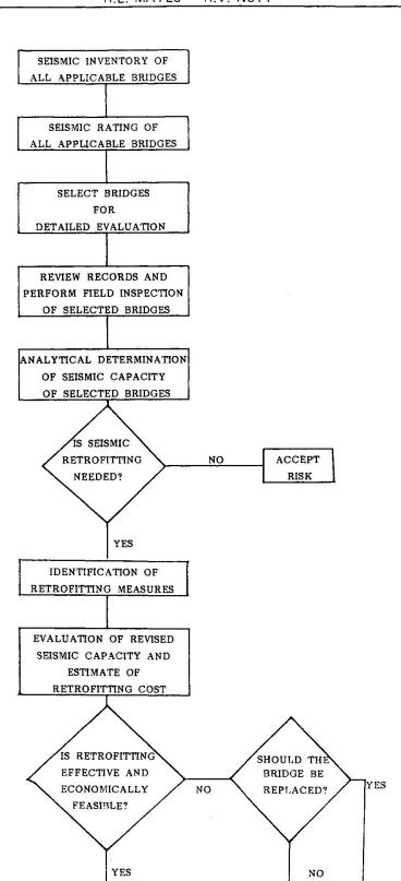
Fig. 2 Seismic retrofitting process for bridges
