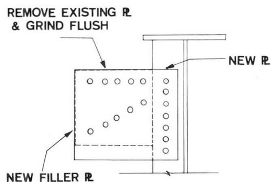
Figure 16 Typical repair
