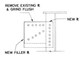
Figure 16 Typical repair
