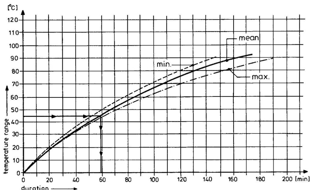
Fig. 7 Duration of temperature Ranges for Insulating Layers
