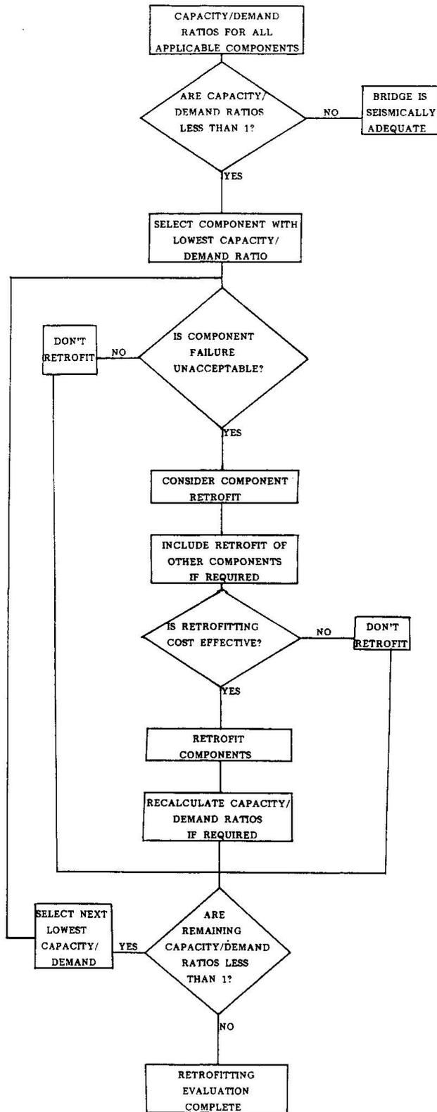
Fig. 3 Procedure for selecting retrofit methods
