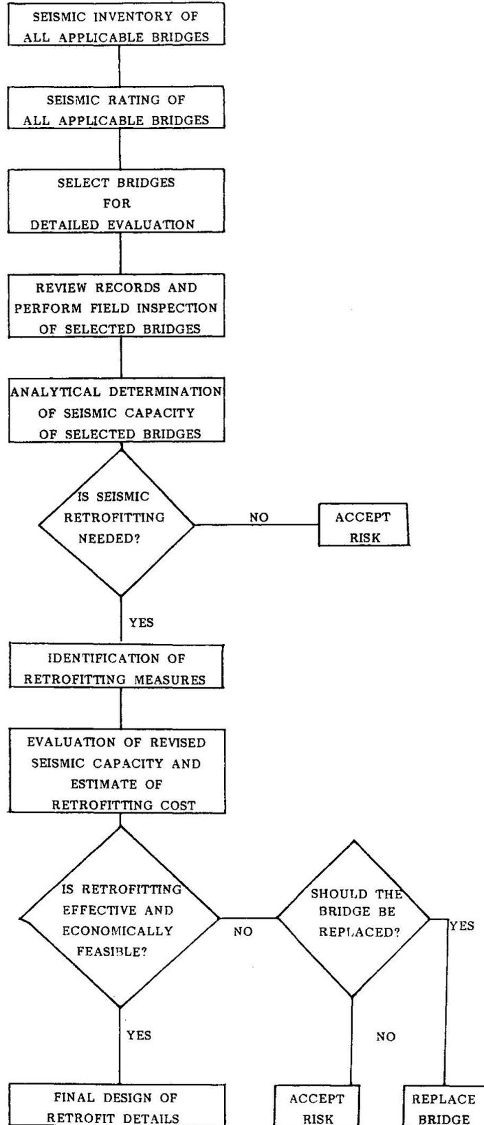
Fig. 2 Seismic retrofitting process for bridges
