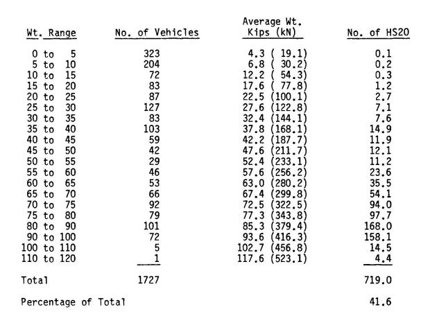
Use of the ADTT data and the DelDOT loadometer data resulted in a calculation of 7.4 million equivalent HS20 vehicles crossing the bridge in 70 years in each direction. This is based on an average ADTT of 2,033 and a projected ADTT of 4,555 at the end of a 70 year life. By comparison, the current AASHTO Specification requires design for 2.0 million cycles (longitudinal members) and over 2.0 million cycles (transverse members) for an ADTT of over 2,500.
