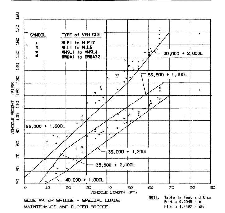
FIGURE 5 - GVW Vs Vehicle Length
