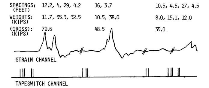
SAMPLE RECORD FROM WIM SYSTEM SHOWING BRIDGE STRAIN OUTPUT, TAPESWITCH SIGNALS AND AUTOMATICALLY PROCESSED TRUCK AXLE AND GROSS WEIGHTS, DIMENSIONS AND SPEEDS [4].
