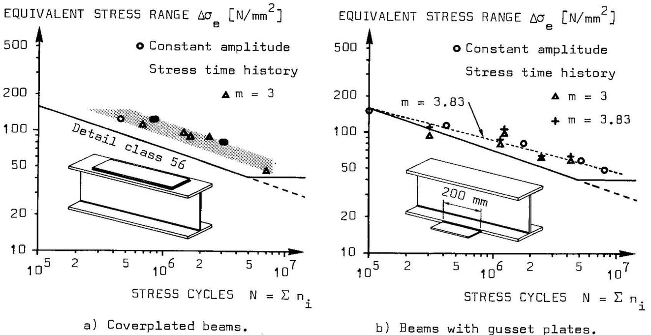
FIGURE 6 : Data from fatigue tests with stress-time histories analyzed by rainflow counting and equivalent stress range (detail class 56 denotes the fatigue strength at  $2 \cdot 10^6$  cycles and is identical to AASTHO category E).
