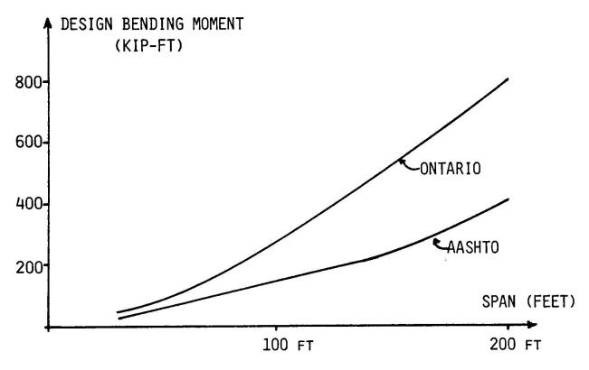
FIGURE 1 COMPARISON OF DESIGN BENDING MOMENTS FOR ONTARIO [9] AND AASHTO [1] BRIDGE SPECIFICATIONS.
