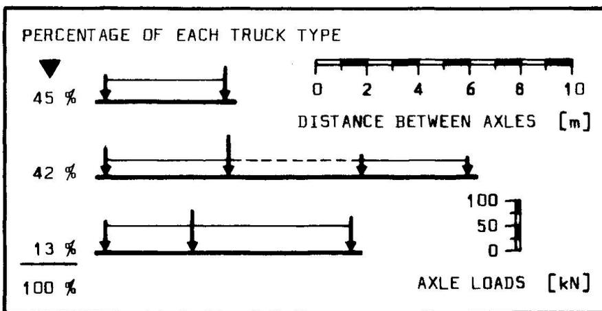
FIGURE 3 : Fatigue load model representing actual traffic on Swiss highway bridges.
