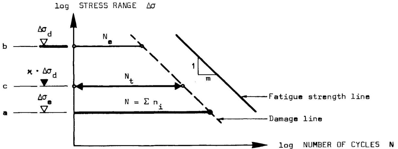
FIGURE 8 : Definition of three levels of stress range with the corresponding number of cycles yielding the same cumulative damage.
