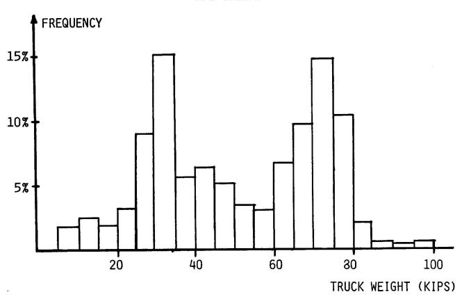
FIGURE 3 SAMPLE WIM GENERATED LOADOMETER SURVEY FOR GROSS TRUCK WEIGHTS [4].
