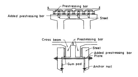
Fig 11 Example of fall-proof device for concrete bridge
