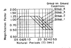
Fig 6 Magnification factor for modified seismic coefficient method
