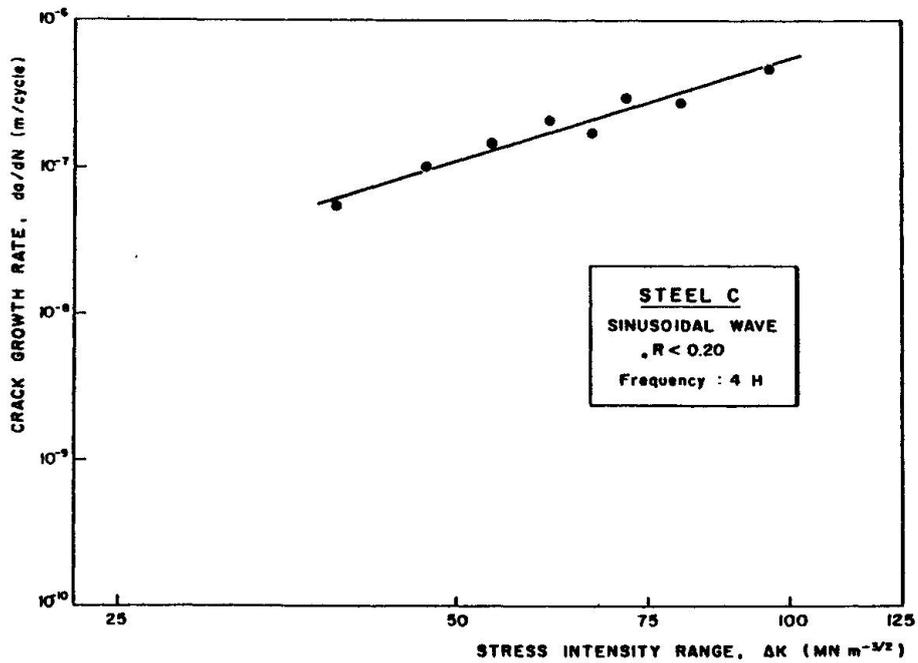
Figure 4. Crack growth rate versus stress intensity range in steel C.
