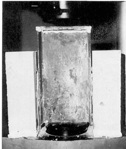
**Fig.3** Typical failure at the interface of the standard specimen
