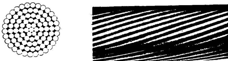
Cable with Helical Wires
